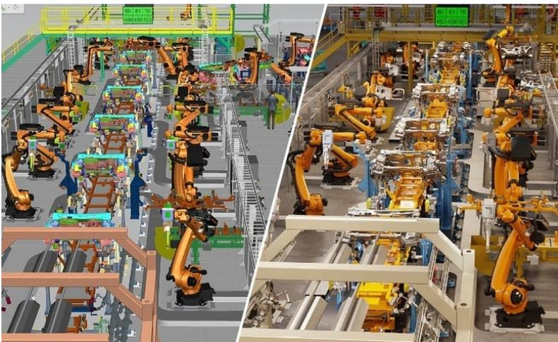
*Figure 1 – A digital twin simulation for demonstrating and validating manufacturing technologies. The vision is for an innovation and demonstration facility with various technologies for multiple users, including OEMs, suppliers, system integrators and equipment builders. Digital twin integration would be one aspect of the ASMIC.*
