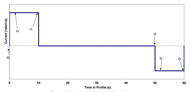
Figure 12. Resistance Calculation Time Points.
