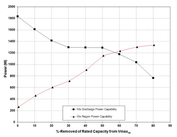
Figure 14. Pulse Power Capability versus %-Capacity Removed.
