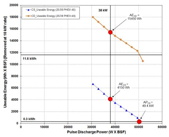
Figure 22. Useable Energy versus Power Curve
