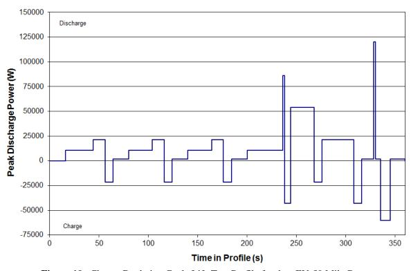
**Figure 10.** Charge-Depleting Cycle Life Test Profile for the xEV-50 Mile Battery.
