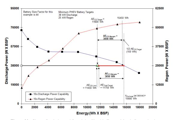
Figure 20. Charge-Depleting and Sustaining Useable Energy Margin Determination.
