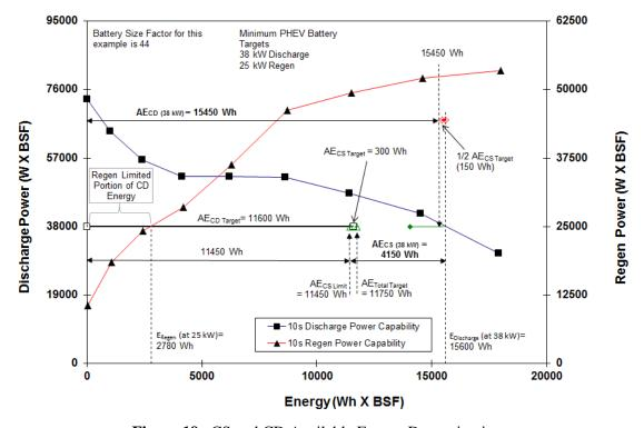
**Figure 19.** CS and CD Available Energy Determination.
