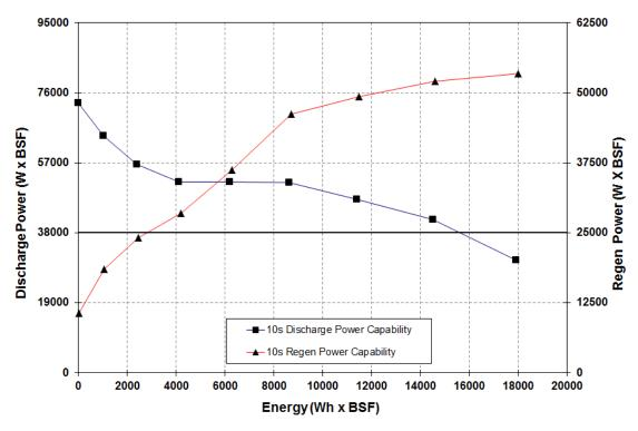
**Figure 17.** HPPC Power vs. HPPC-Current Discharge Energy Scaled by the Battery Size Factor.
