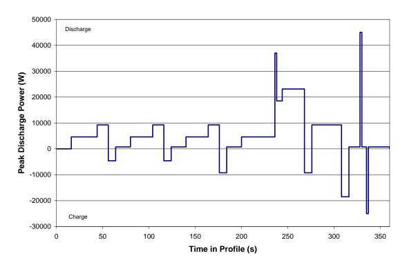
**Figure 8.** Charge-Depleting Cycle Life Test Profile for the PHEV-20 Mile Battery.
