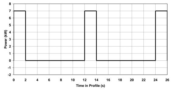
Figure 4. Cold Cranking Test Profile.
