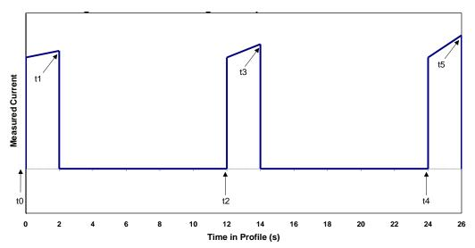
Figure 26. Cold Cranking Test Resistance Calculation Points.
