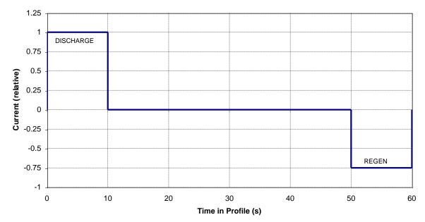
Figure 1. Hybrid Pulse Power Characterization Test Profile.
