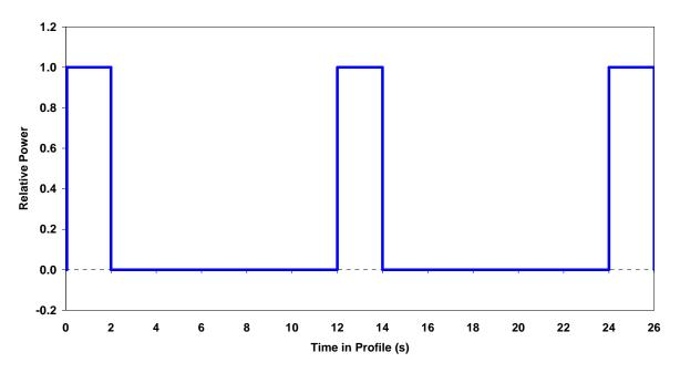
Figure 4. Cold Cranking Test Profile
