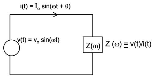
Figure 1C. Experimental setup for EIS measurements.
