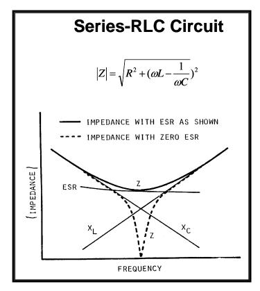
Figure 3C. Magnitude of the impedance as a function of frequency.
