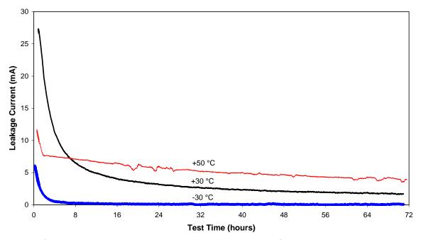
Figure 12. Leakage current measured on a capacitor at three temperatures.
