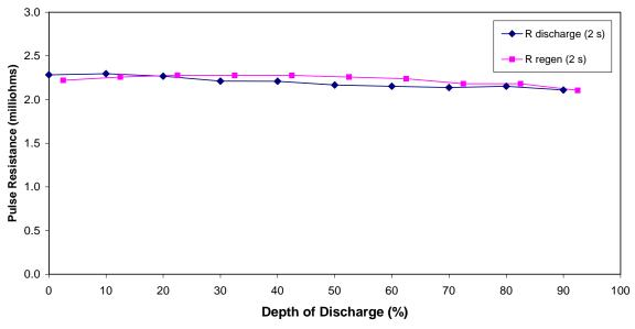
Figure 21. Discharge and Regen Pulse Resistances for an HPPC Test
