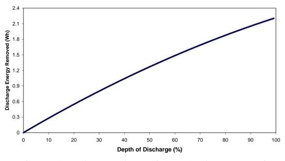
Figure 19. Energy from the Reference Discharge Test for a Representative Capacitor
