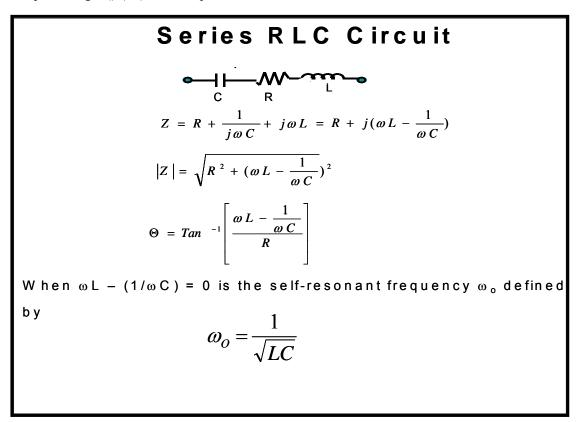
Figure 2C. Series RLC circuit model for a two terminal device.
