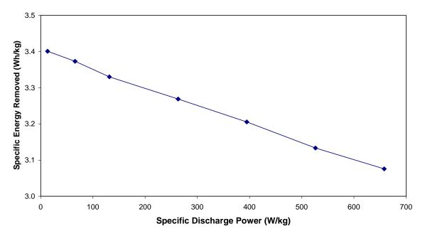
Figure 11. Specific Energy versus Specific Power for a Representative Ultracapacitor
