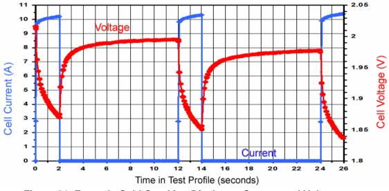
Figure 31. Example Cold Cranking Discharge Current and Voltage
