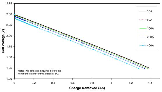
Figure 7. Cell voltage as a function of charge removed for a series of constant-current tests.
