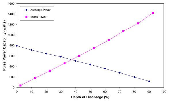
Figure 23. Example Pulse Power Capability Results from an HPPC Test
