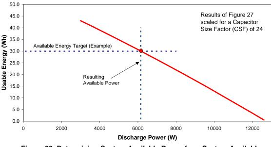
Figure 28. Determining System Available Power for a System Available Energy Goal of 30 Wh with CSF = 24
