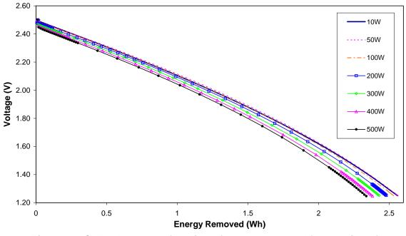
Figure 10. Cell voltage as a function of energy removed for a series of constant-power discharge cycles.
