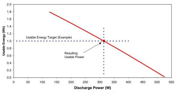
Figure 27. Determination of Usable Power at a Selected Usable Energy Target
