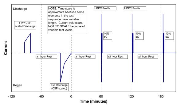
Figure 2. Start of HPPC Test Sequence
