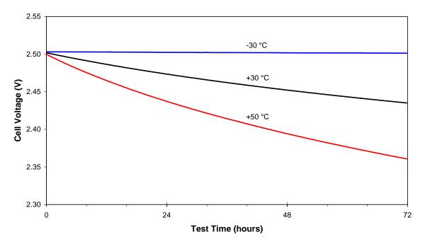
Figure 15. Cell voltage during a Self-Discharge Test measured at several temperatures.
