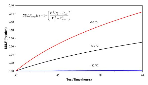
Figure 16. Self-Discharge Energy Loss Factor calculated from the data of Figure 15.
