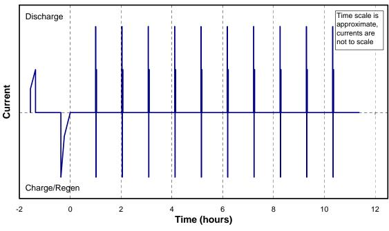
Figure 3. Complete HPPC Test Sequence
