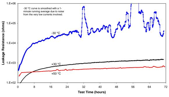
Figure 13. Leakage resistance determined from data in Figure 12 for a capacitor at three temperatures.
