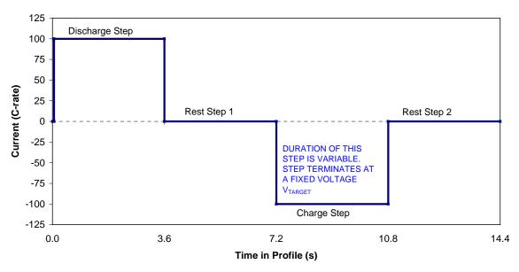
Figure 5. Ultracapacitor Energy Efficiency and Life Test Profile
