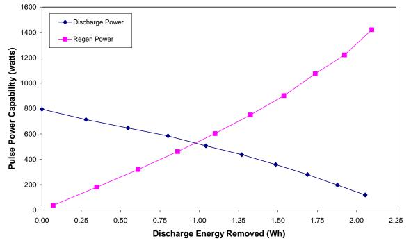
Figure 24. HPPC Power Capability versus Energy Removed for the data presented in Figures 19 and 23 (unscaled).
