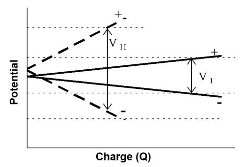
**Figure A-2.** Electrode potentials for an aqueous symmetric Generation I (solid) and an organic symmetric Generation II (dashed) electrochemical capacitor during application of charge Q.
