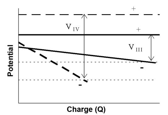
**Figure A-3.** Electrode potentials for a Generation III (solid) and Generation IV (dashed) electrochemical capacitor during application of charge Q.
