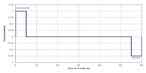
Figure 1. Ultracapacitor HPPC Test Profile
