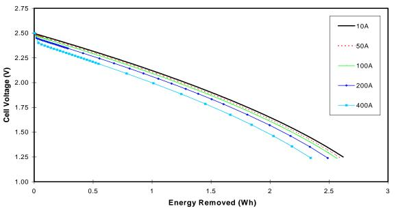
Figure 8. Cell voltage as a function of the energy removed for a series of constant-current tests.
