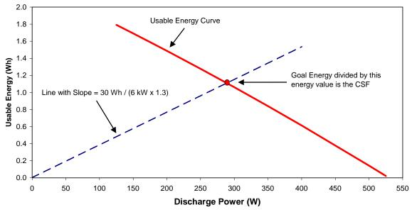
Figure 29. Finding a Capacitor Size Factor Using Device-Level Results.
