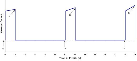
Figure 30. Cold Cranking Resistance Calculation Points
