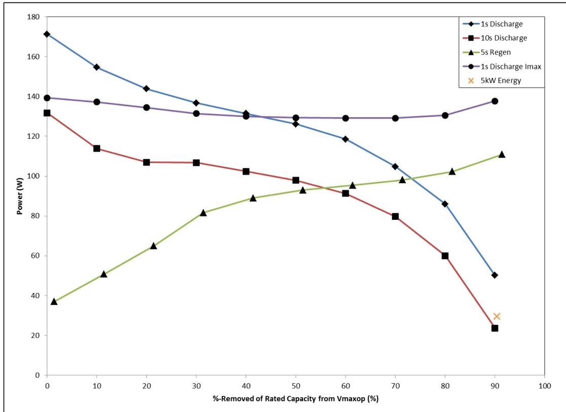
**Figure 9.** Pulse power capability vs depth of discharge.
