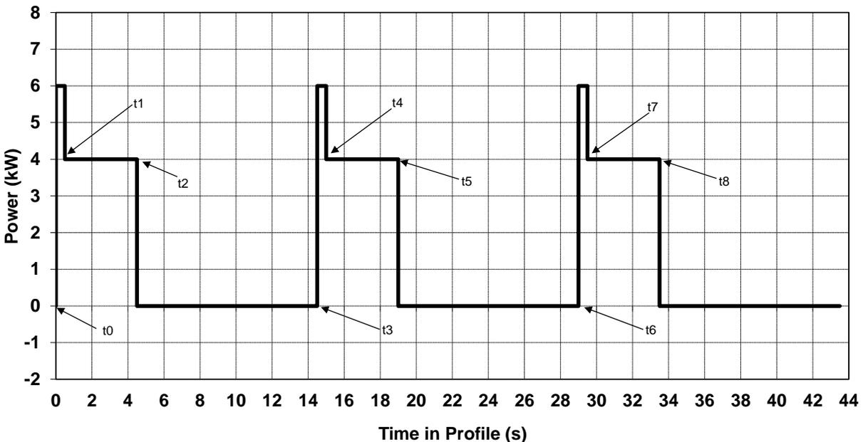
**Figure 19.** Cold Cranking Test resistance calculation points.
