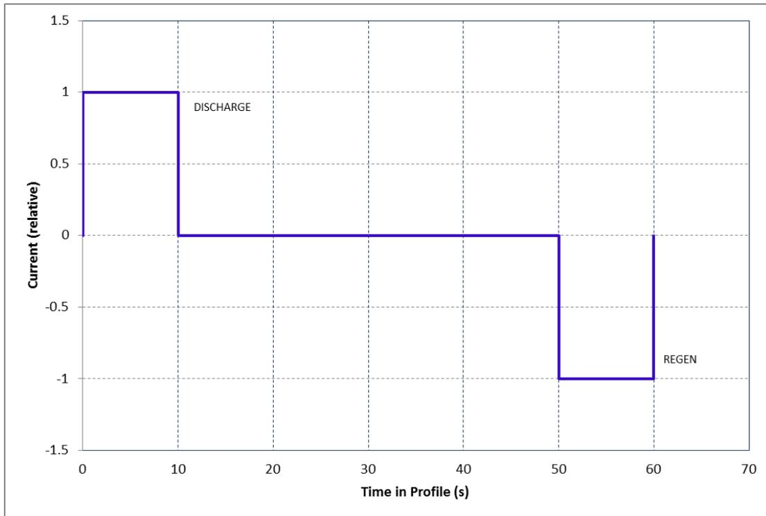
**Figure 1.** Hybrid Pulse Power Characterization Test profile.
