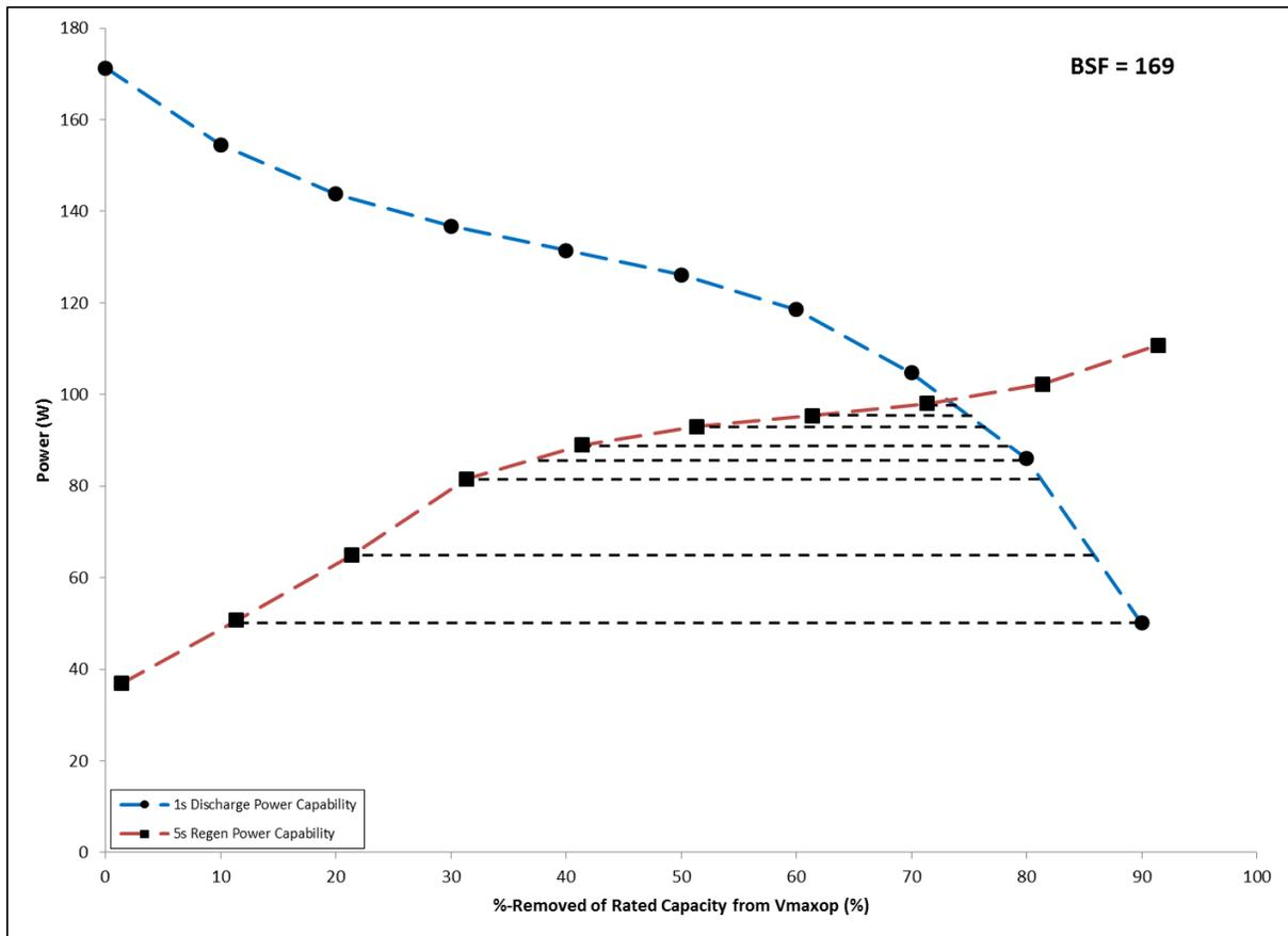
**Figure 17.** Finding the Useable Energy Using Device-Level Results.
