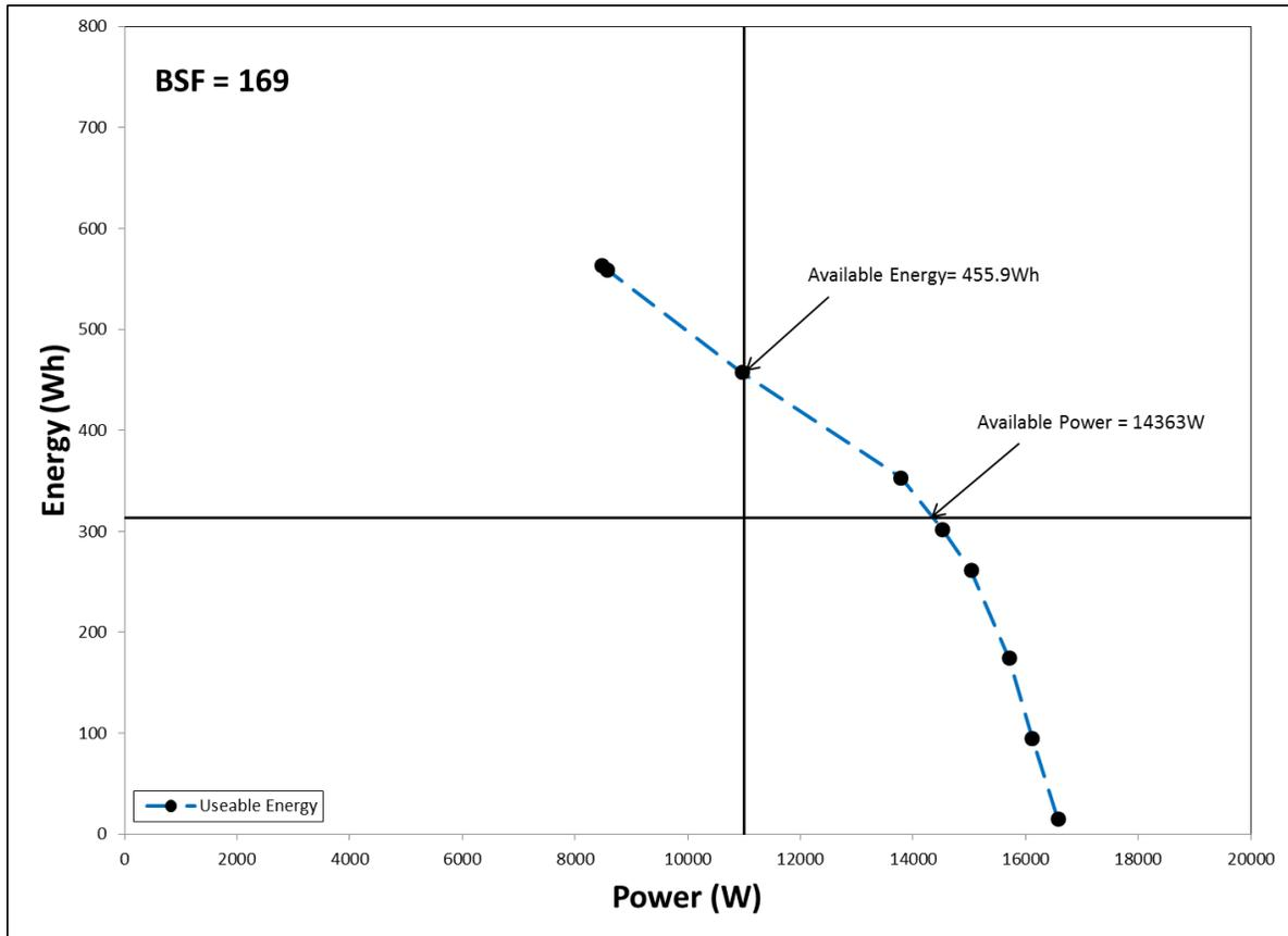
**Figure 15.** Useable Energy versus Power Curve.
