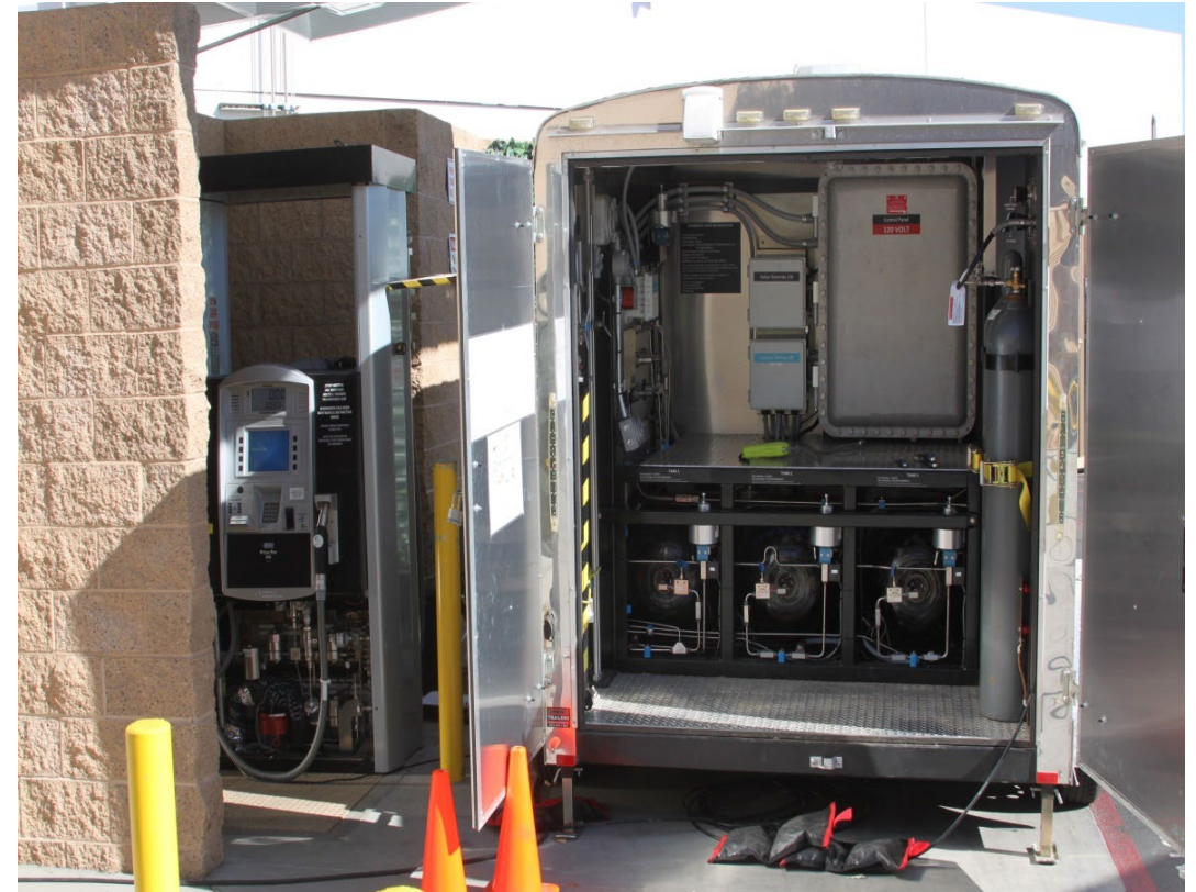
Light-duty HyStep Trailer shown above, used to evaluate the hydrogen station capability to fill according to the J2601 requirements. Similar devices and tools are being developed for medium-duty and heavy-duty hydrogen stations.
