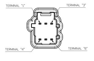
CONNECTOR PIN OUT (SCALE 2:1)
