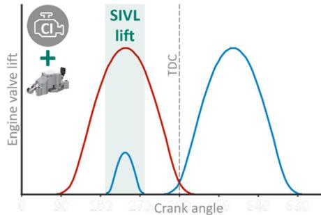
Secondary intake valve lift for CI EGR control
