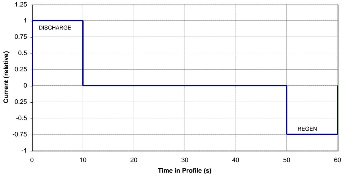
**Figure 1.** Hybrid Pulse Power Characterization Test Profile.
