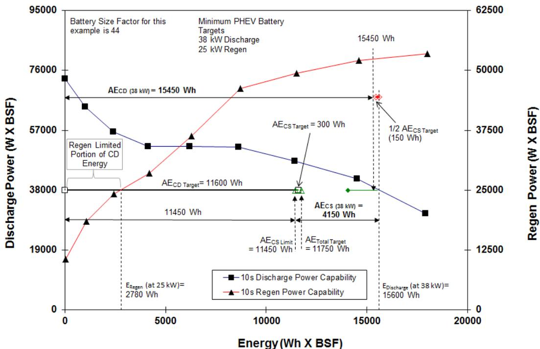
Figure 19. CS and CD Available Energy Determination.
