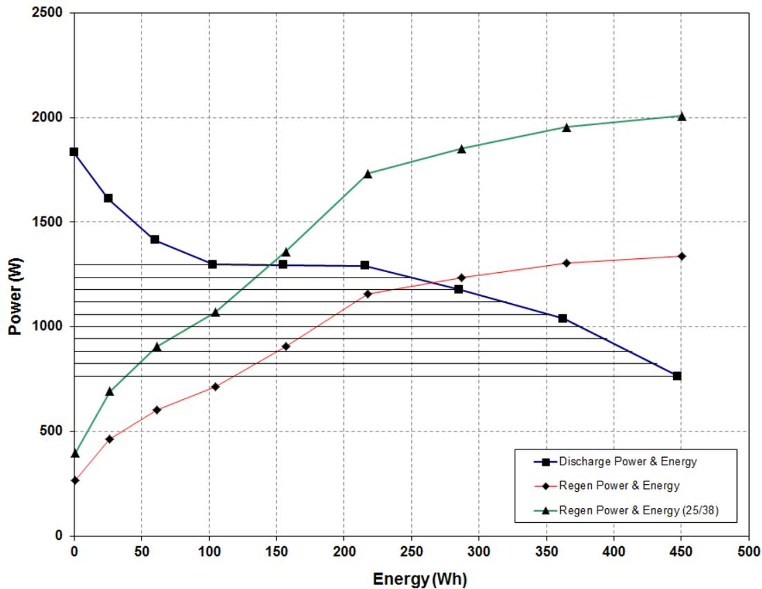
**Figure 24.** Finding the Useable Energy Using Device-Level Results.
