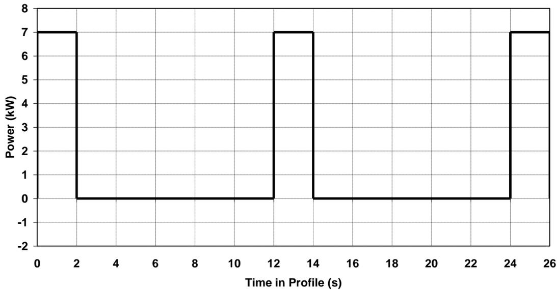
**Figure 4.** Cold Cranking Test Profile.
