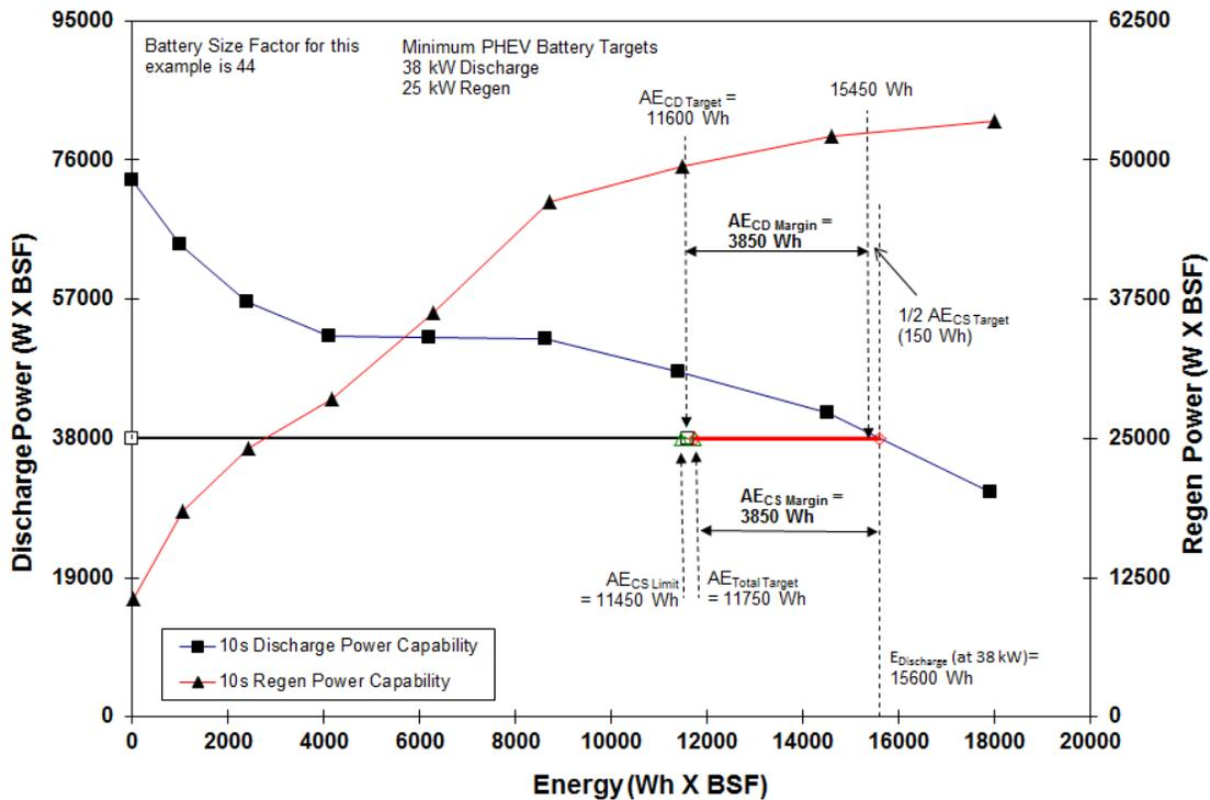
Figure 20. Charge-Depleting and Sustaining Useable Energy Margin Determination.
