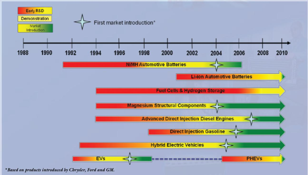
This chart shows the progress of U.S. Government/USCAR collaborative R&D to advance key automotive technologies. The stars indicate when those technologies were first introduced in U.S. production vehicles. The chart also shows new technologies that continue to be developed, including some for which market introduction is imminent.
