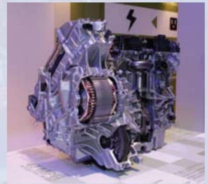
The 2010 Ford Fusion Hybrid Electric Motor Cutaway
