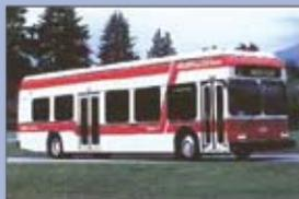
Phase II Ballard hydrogen fuel cell bus
