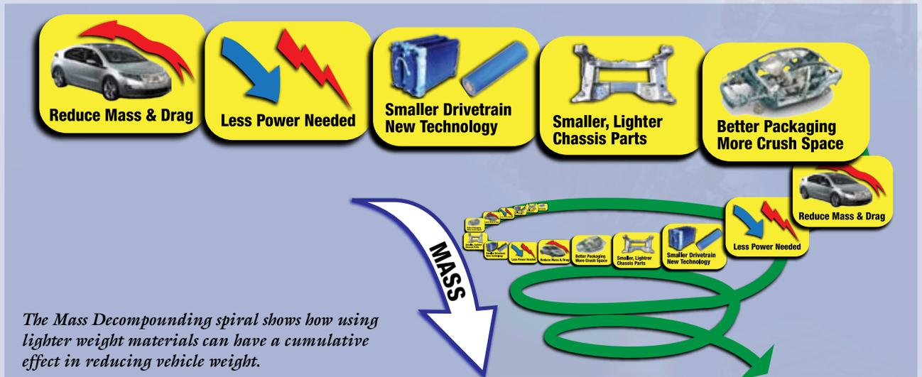
*The Mass Decomponding spiral shows how using lighter weight materials can have a cumulative effect in reducing vehicle weight.*
