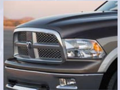
The 2010 Dodge RAM 1500 utilizes an aluminum hood and components to reduce vehicle weight.
