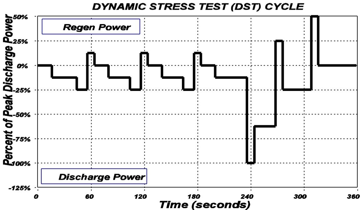
Figure 5B-1. DST Profile in Relative Power Units
