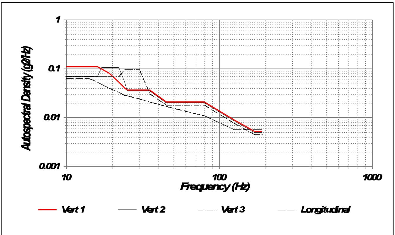
Figure 1. Vibration Spectra for Random Vibration Test
