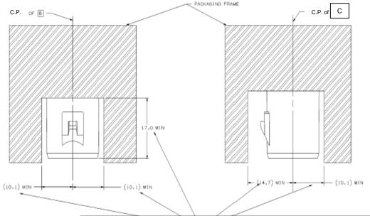
If header is recessed into a pocket, these dimensions represent the minimum clearance required for the mating connector shroud. Note: Additional clearance may be required to allow latch function.
