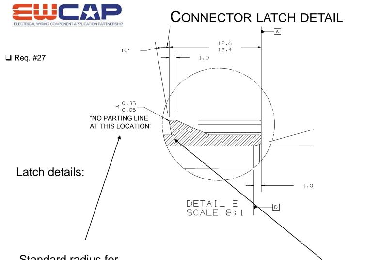
Standard radius for back of external lock (prevents flash and possible lock arm hang-up). No parting line allowed here
