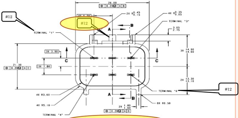
Label the corner blade locations as shown. The interface primary view is to be oriented with the latch feature at the top, looking into the footprint at the tips of the male blades, number 1 is in the upper left corner. The last number position is the lower right in the field. Each row of terminals are numbered left to right. Follow USCAR-12 Appendix A for non-standard terminal layouts. Blade center planes must be per the EWCAP guidelines unless an engineering reason exists for a variance..
