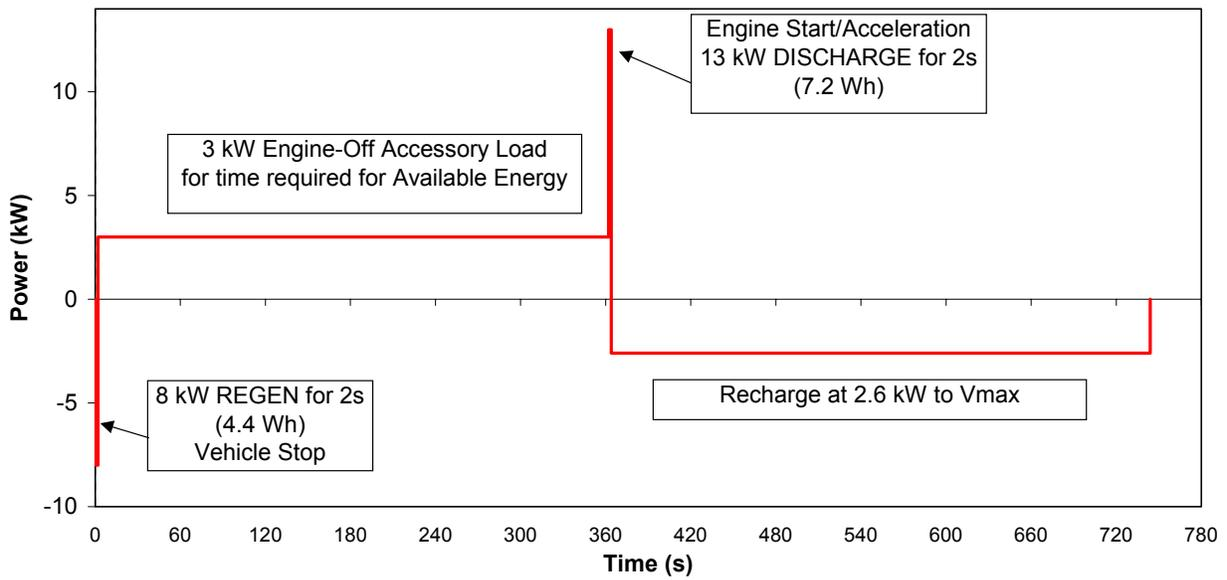
**Figure 3.** M-HEV Power & Energy Design Verification Load Profile
