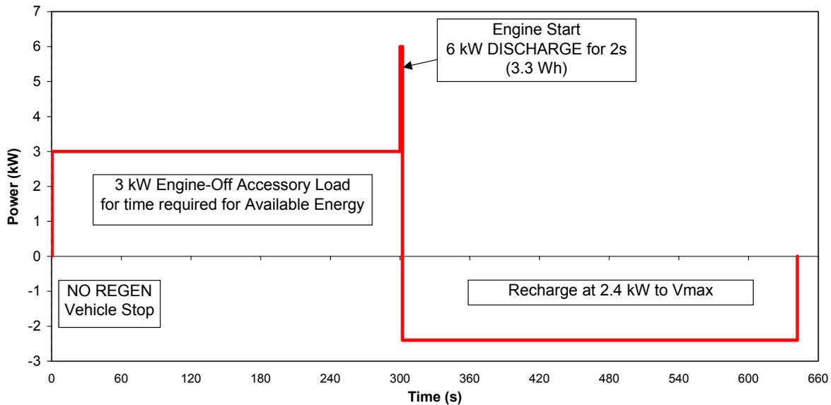
**Figure 2.** Start-Stop Power & Energy Verification Design Load Profile
