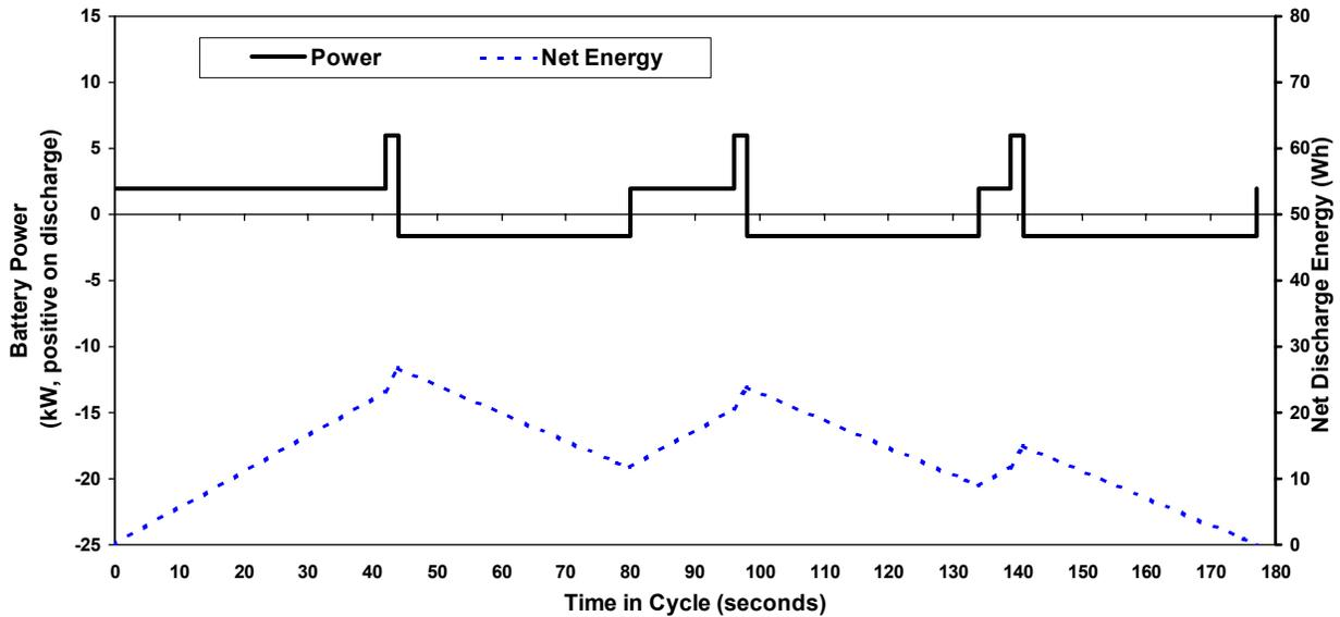
**Figure 8.** Zero Power-Assist (ZPA) Efficiency and Life Test Profile
