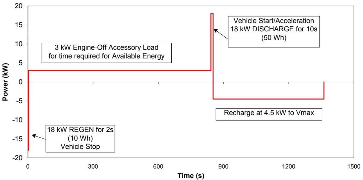
**Figure 4.** P-HEV Power & Energy Design Verification Load Profile
