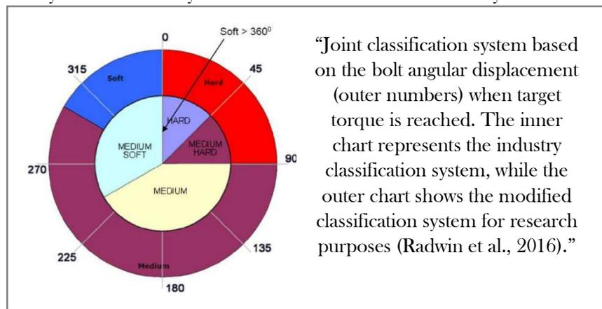
Figure 2. Hard and soft joint specifications
