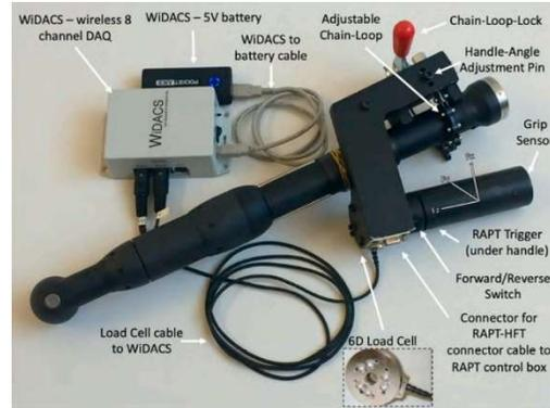
Figure 1. RAPT-FH: Instrumented tool for RAPT hand force measurement
