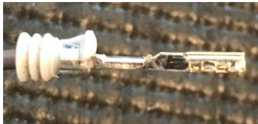
FIGURE 4.2.5J – EXCESSIVE CABLE SEAL NECK
