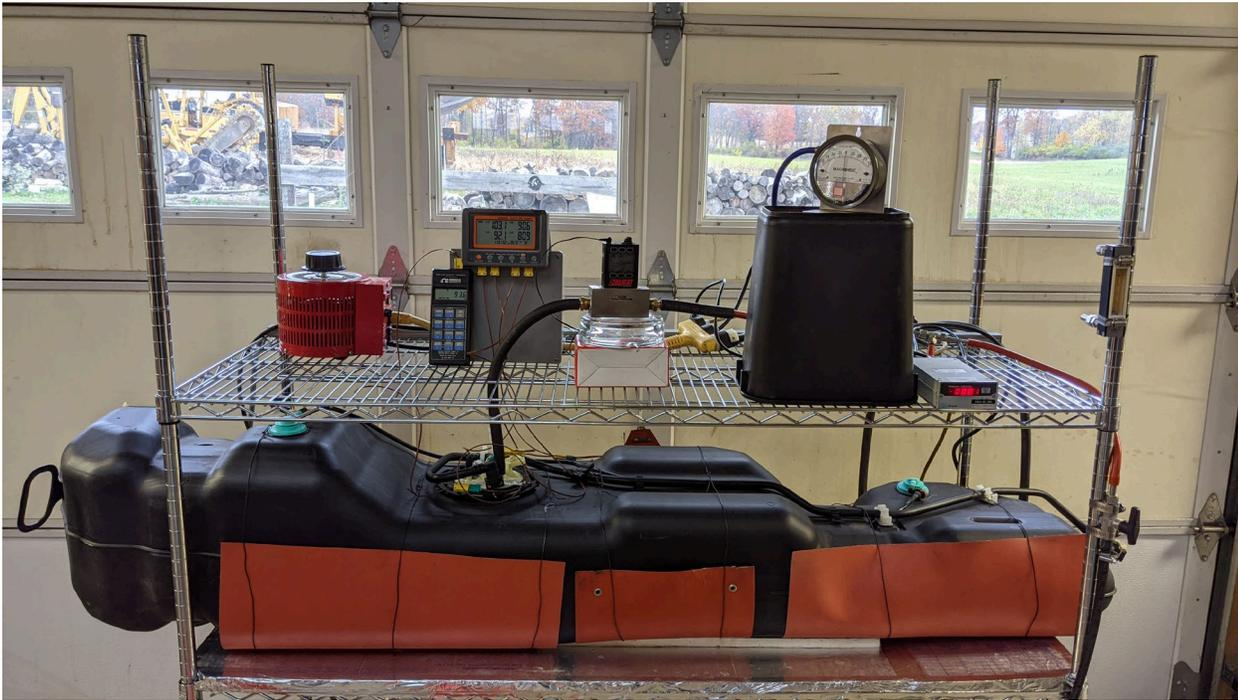
During the experiment the fuel tank was wrapped in a blanket to keep the temperature around the tank constant (simulating an on-road environment), and the entire setup, which was installed on a metal rack on wheels, was gently moved back and forth every five minutes to ensure good mixing and constant heat distribution through the fuel as it would in an actual vehicle on-road in use.
