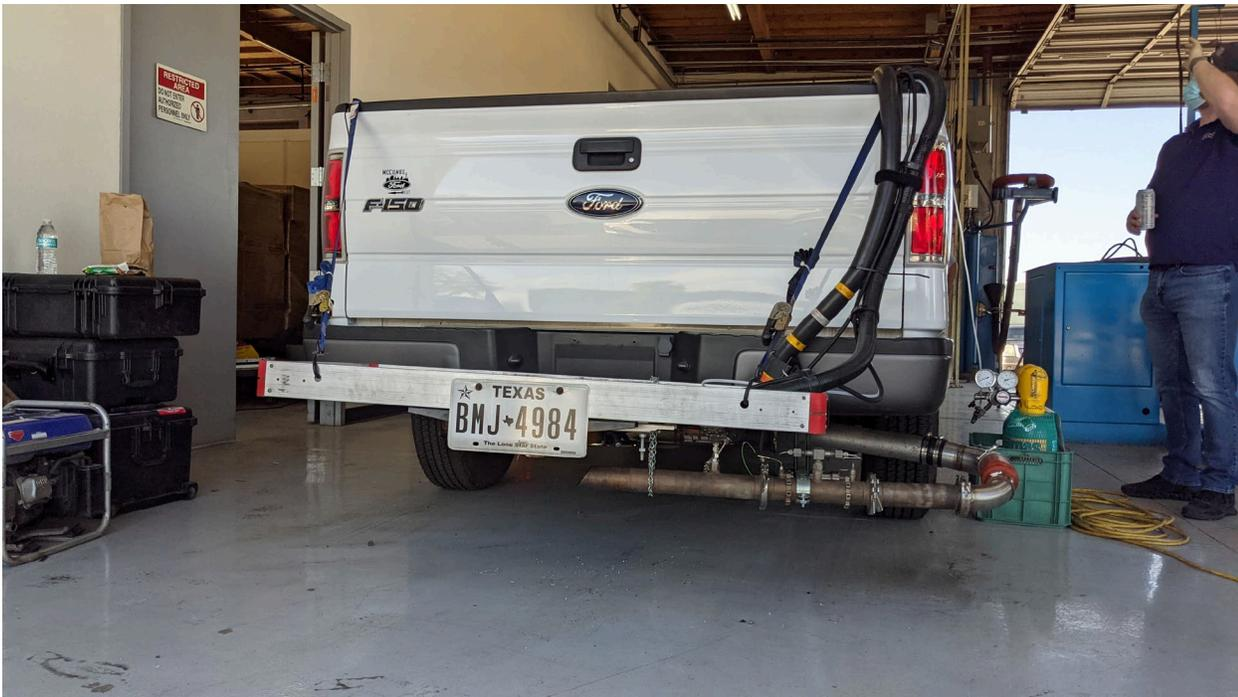
**Picture 16 - F-150 with PEMS Installed Ready for Data Collection**
