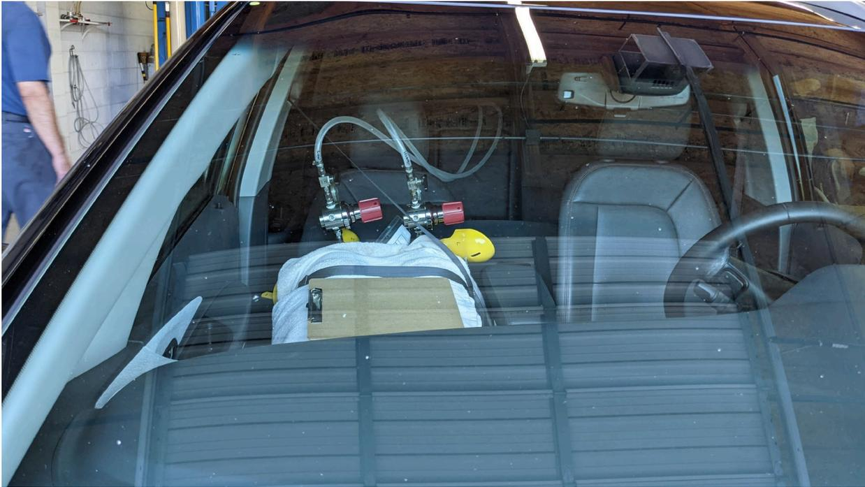
**Picture 31 - Electric Vehicle With Simulated Tailpipe Installed**
