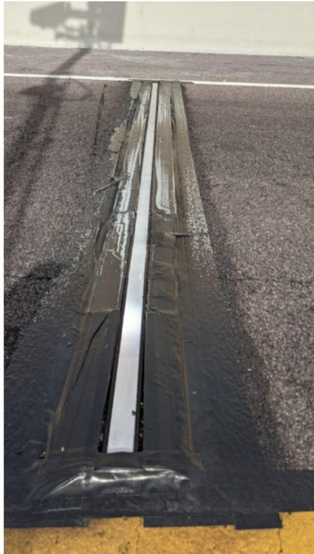
**Pictures 24 - HEAT EDAR System, Retroreflector on-road and Opus Sensor Approximately 9 Feet Away (Day 1 Of Study)**
