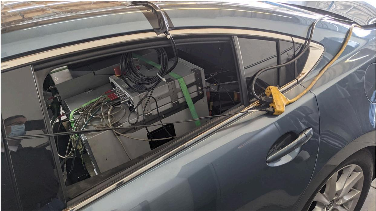
Picture 18 - Mazda6 with PEMS Sampling System Being Installed
