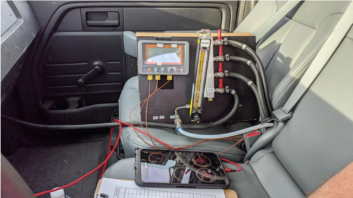
**Picture 9 - Control Board in Mazda6 with Butane Tank**
