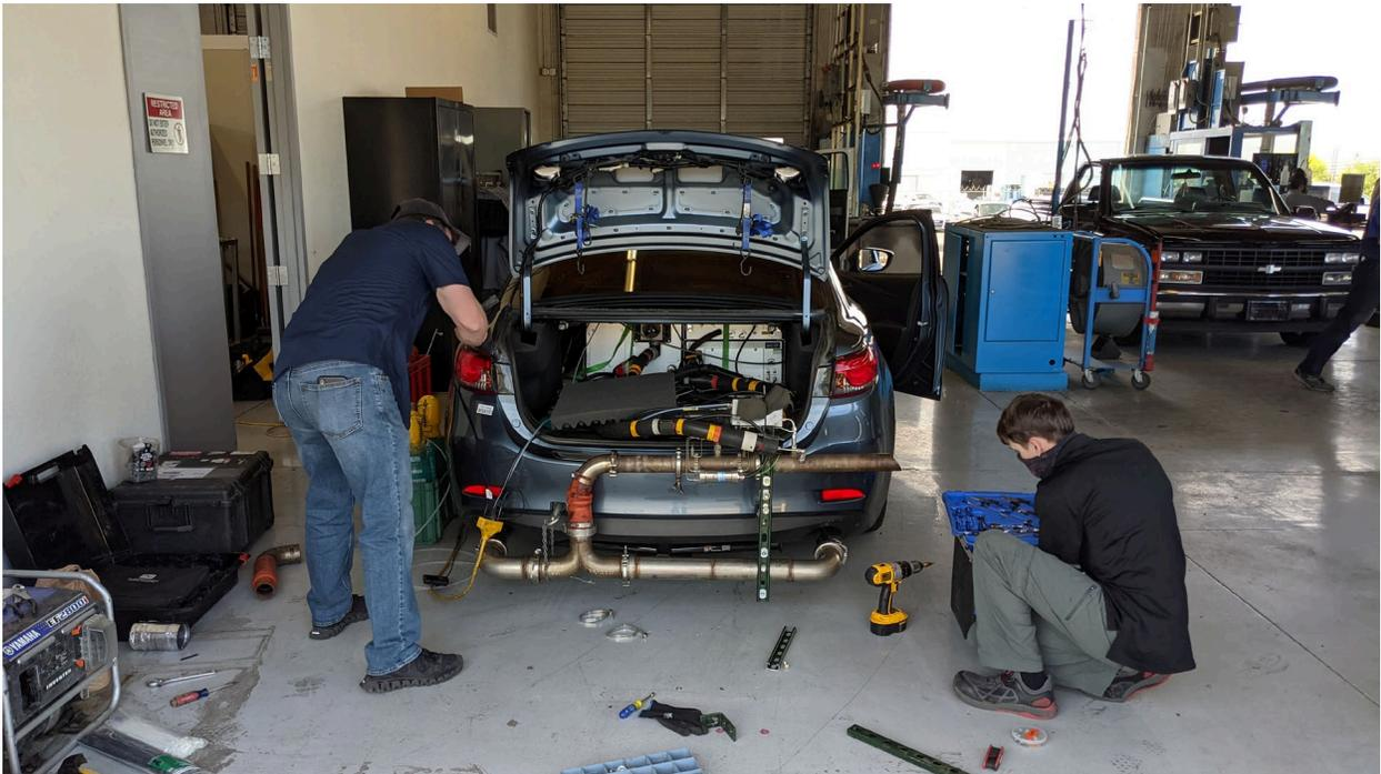
**Picture 19 - Mazda6 with PEMS Installed Ready for Data Collection**
