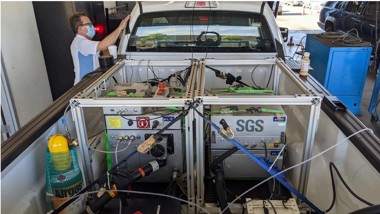
Picture 15 - Exhaust Sampling and Flow Measurement For F-150 PEMS
