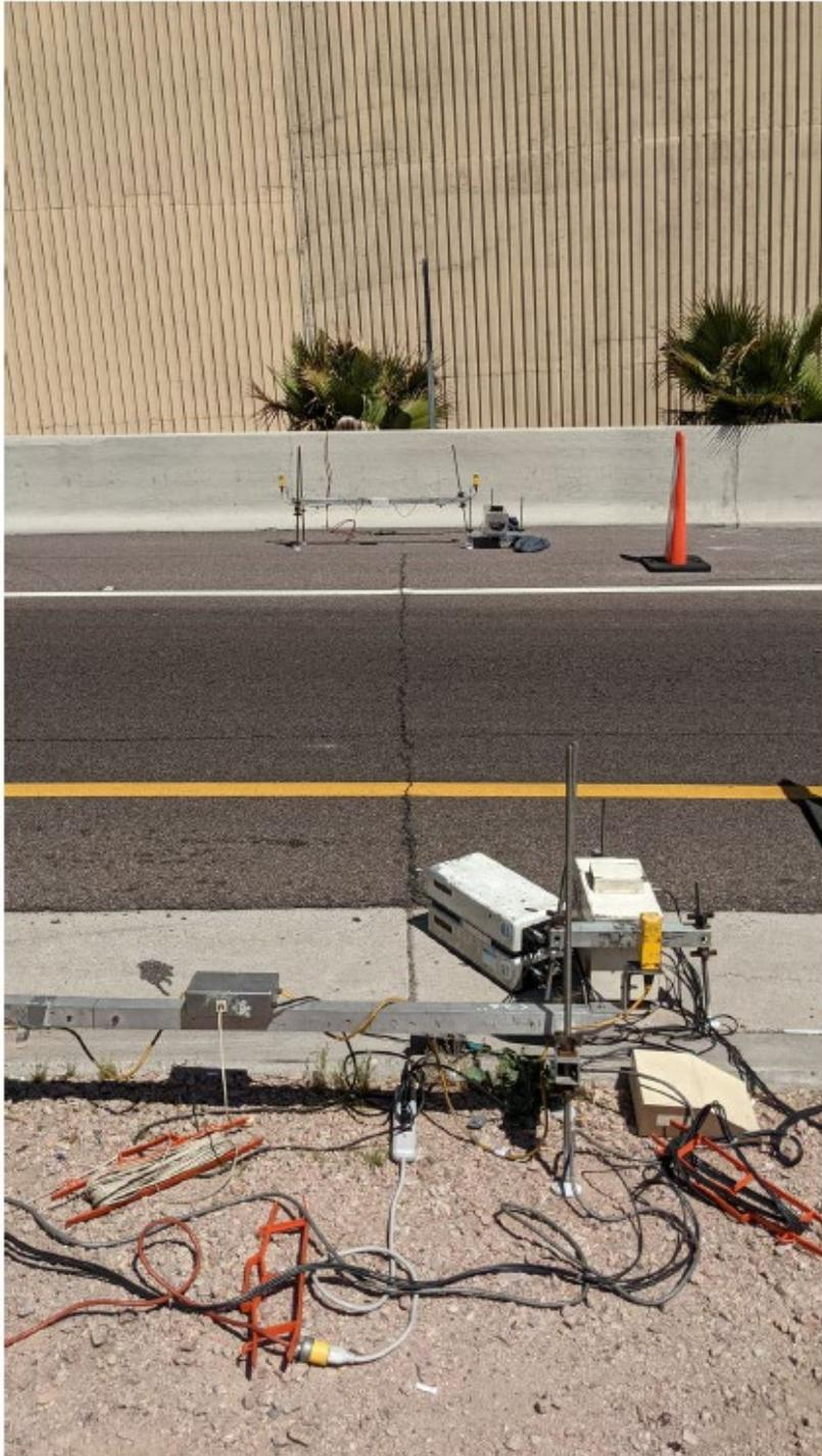
Picture 29 - DU FEAT Data Capture, License Plate Picture and Analysis Computer
