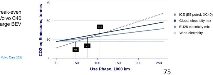
Emissions break-even diagram for Volvo C40 Recharge BEV
