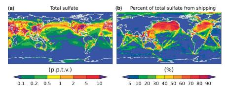
Total sulfate (parts per trillion by volume) and percentage of total sulfate provided by shipping prior to IMO regulations on sulfur content of fuels
