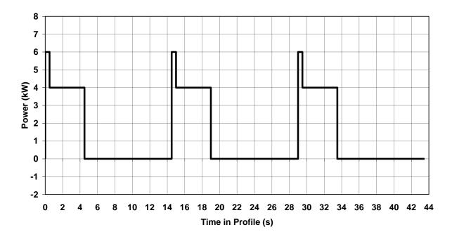
Figure 4. Cold Cranking Test profiles.
