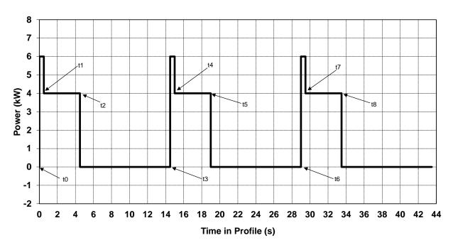
Figure 19. Cold Cranking Test resistance calculation points.
