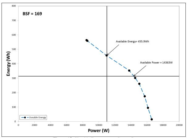
Figure 15. Useable Energy versus Power Curve.
