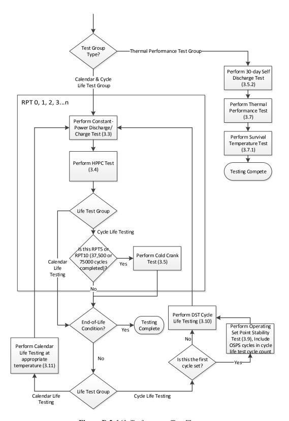
Figure D.2. Life/Performance Test Flow
