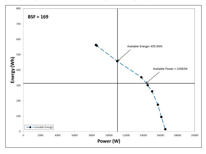
Figure B.2. Useable Energy Versus Power Curve
