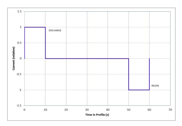
Figure 1. Hybrid Pulse Power Characterization Test profile.
