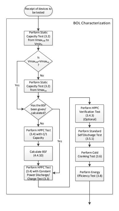
Figure D.1. Beginning of Life Characterization Test Flow
