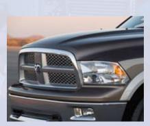
The 2010 Dodge RAM 1500 utilizes an aluminum hood and components to reduce vehicle weight.
