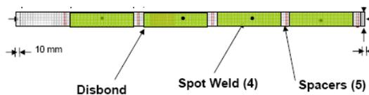
An example of the coupons prior to assembly is shown in Figure 1 showing the wire spacers used to control the adhesive thickness, intentional skips,
