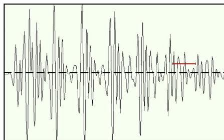
Figure 11: Representative Pulse/echo Signals on a Test Specimen – Adhesive Present.
