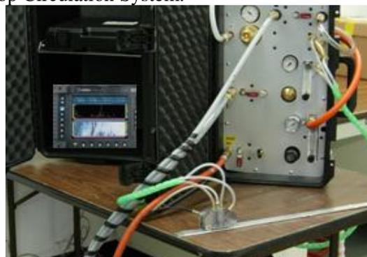
The holder uses a closed-loop water circulation system to maintain a water column between the array and the flange surface. The angled inlet port (Figure 4) supplies the water below the array while the two vertical ports vacuum excess water from the part. The closed-loop circulation system was designed and built to include a filtered water supply, return pump and coupling gages in a self contained shipping case (Figure 5).
