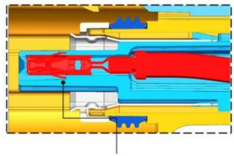
Terminal tangs, lock finger, and independent secondary lock must provide all the terminal retention for 110N criteria to apply (i.e. ferrule cannot contribute to terminal retention).
