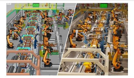
**Figure 1** – A digital twin simulation for demonstrating and validating manufacturing technologies. The vision is for an innovation and demonstration facility with various technologies for multiple users, including OEMs, suppliers, system integrators and equipment builders. Digital twin integration would be one aspect of the ASMIC.
