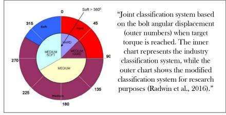
Figure 2. Hard and soft joint specifications
