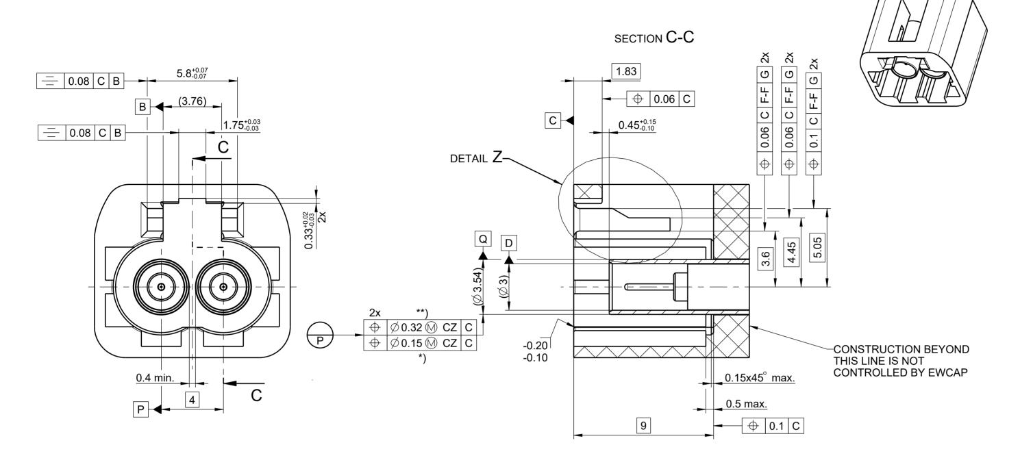
\*) THE SPECIFIED DEVIATION APPLIES ONLY FOR PCB-PLUG, REFERRING TO MEASURING PLANE 1.
