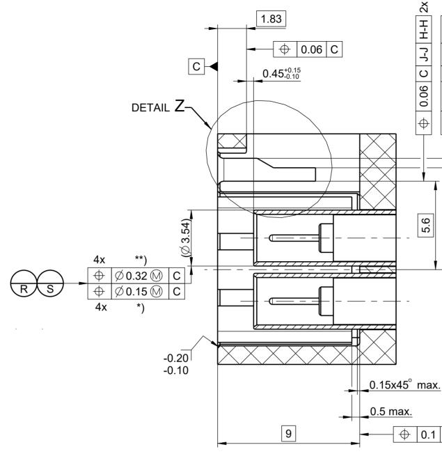
\*) THE SPECIFIED DEVIATION APPLIES ONLY FOR PCB-PLUG, REFERRING TO MEASURING PLANE 1. \*\*) ONLY VALID FOR FLOATING OUTER CONTACT OF THE CABLE PLUG, REFERRING TO MEASURING PLANE 1.
