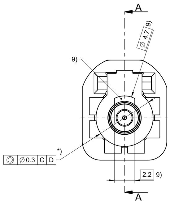
\*) FOR FLOATING OUTER CONTACT OF THE CABLE PLUG, A DEVIATION OF  $\varnothing 0.4$  IS PERMISSIBLE, REFERRING TO MEASURING PLANE 1.
