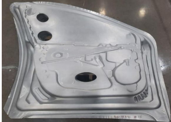
Figure G3.8: Door Inner: A good quality part and final forming process parameters. (Source: Promatek)
