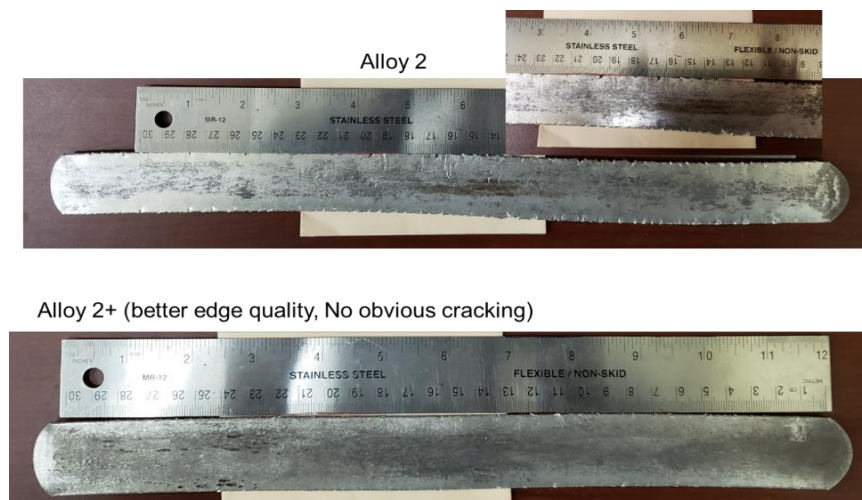
Figure C6.4: Alloy 2 and Alloy 2 Plus sheets rolled to large reductions at 275°C. (Source: ORNL)
