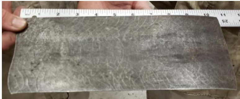
Figure C6.1: Rolled Alloy 2 Plus sheet, 1.65 mm thick, 110 mm wide. (Source: ORNL)
