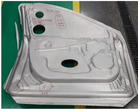
Figure G3.6: Door inner: Initial tryout stamping with splits and wrinkles, and process parameters. (Source: Promatek)
