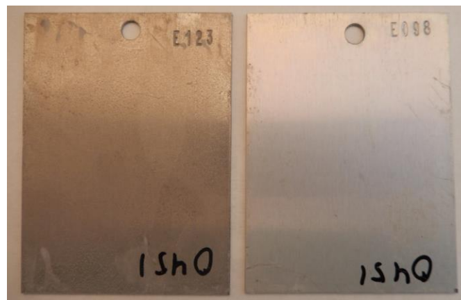
Figure D1.2. EFP panels after 24-hour humidity exposure. (left) Control panel (solvent cleaned only). (right) Panel having Henkel pretreatment C. (Source: Henkel)
