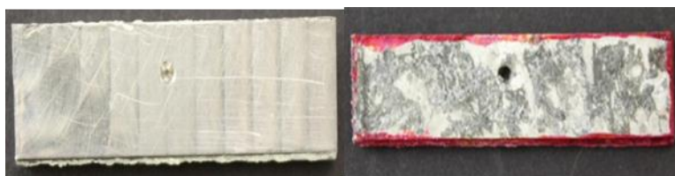
Figure D2.2: AZ31B samples, 15 x 50 mm. (left) As-received and (right) after 48 hours of ASTM B117 salt fog. (Source: Xtalic)
