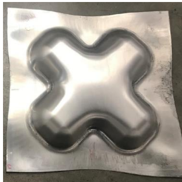
Figure G2.1: Warm-stamped cross-form, approximately 470 mm square. (Source: EWI)
