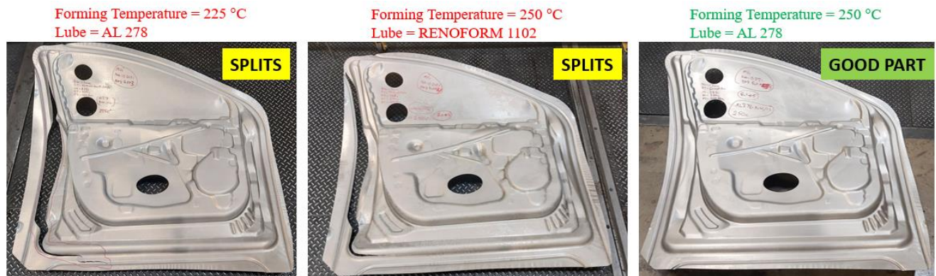
Figure G3.3: Door inner forming results illustrating effect of temperature and lubricant selection. (Source: Promatek)
