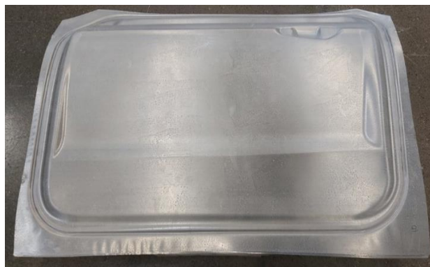
Figure G3.5. Door outer: A good quality panel and associated final forming process parameters.
