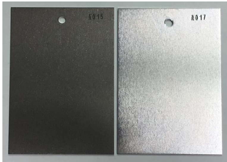
Figure D1.1: ZEK100 sheet before (left) and after (right) deoxidation (Source: Henkel)
