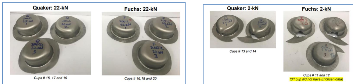
Figure G1.1: Examples of Good (left) and Bad (right) drawn cups. (Source: EWI)
