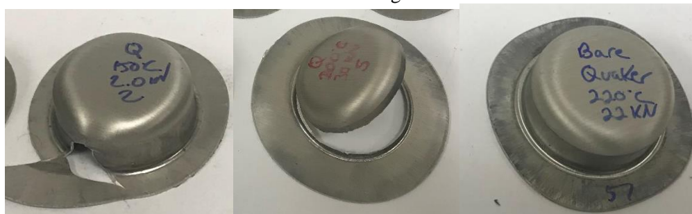
Figure D4.4: Cup draw test samples. EFP sheet blanks with Quaker 450 lubricant applied. (a) 150°C, 2-kN BHF and (b) 200°C, 30-kN BHF. (c) Crack-free and formed to full depth using 220°C, 22-kN BHF. (Source: Quaker)
