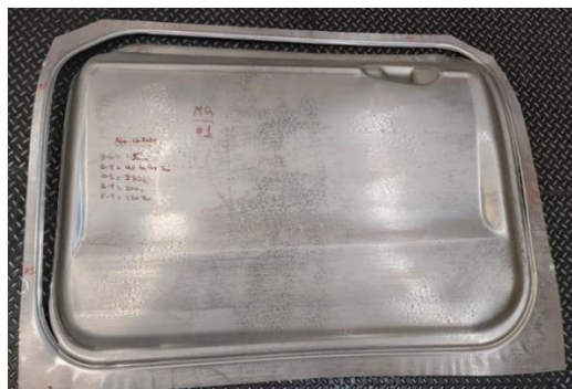
Figure G3.4: Door outer: Badly split initial tryout stamping and associated process parameters. (Source: Promatek)
