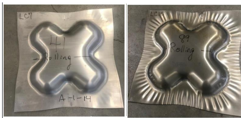
Figure G1.4: Examples of (left) Good and (right) Bad EFP cross-forms stampings. (Source: EWI)
