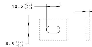
0.6mm to 4.0mm Thickness to be agreed between supplier and customer USCAR-44 Table 5.3.2 should be consulted for related testing
