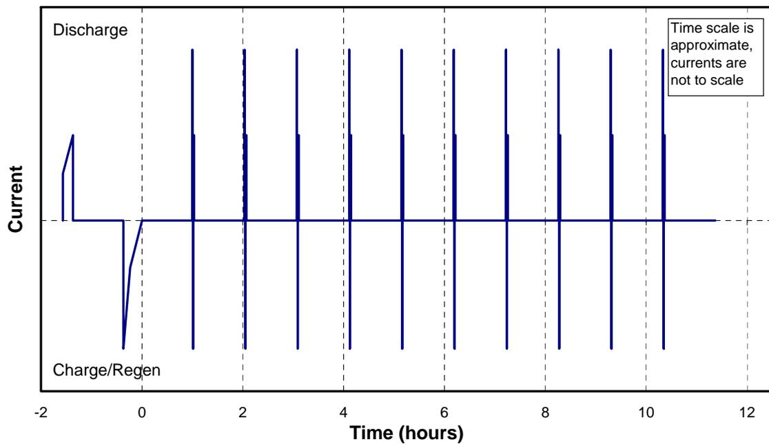
Figure 3. Complete HPPC Test Sequence
