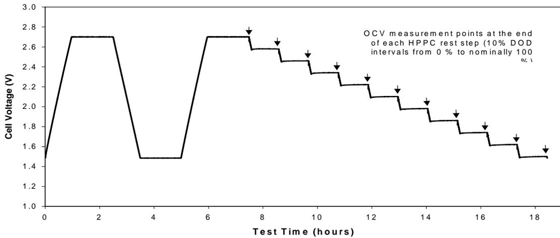
Figure 17. Capacitor Voltage versus Time for an Example HPPC Test
