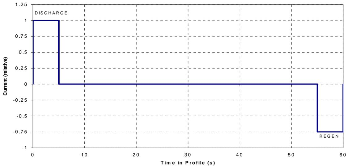
**Figure 1. Ultracapacitor HPPC Test Profile**
