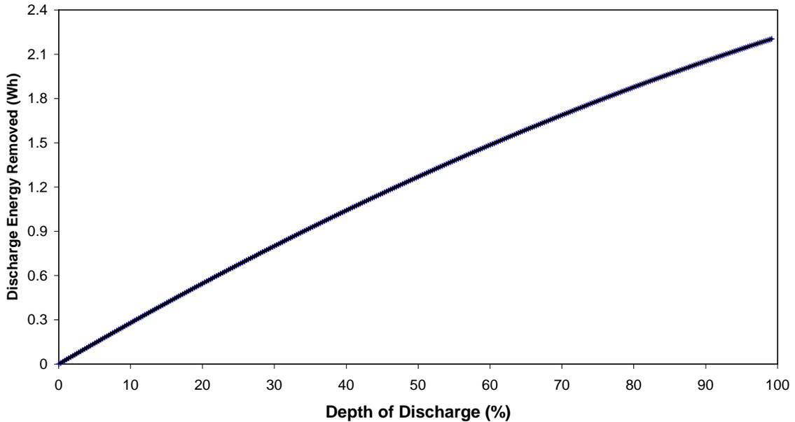
**Figure 19. Energy from the Reference Discharge Test for a Representative Capacitor**
