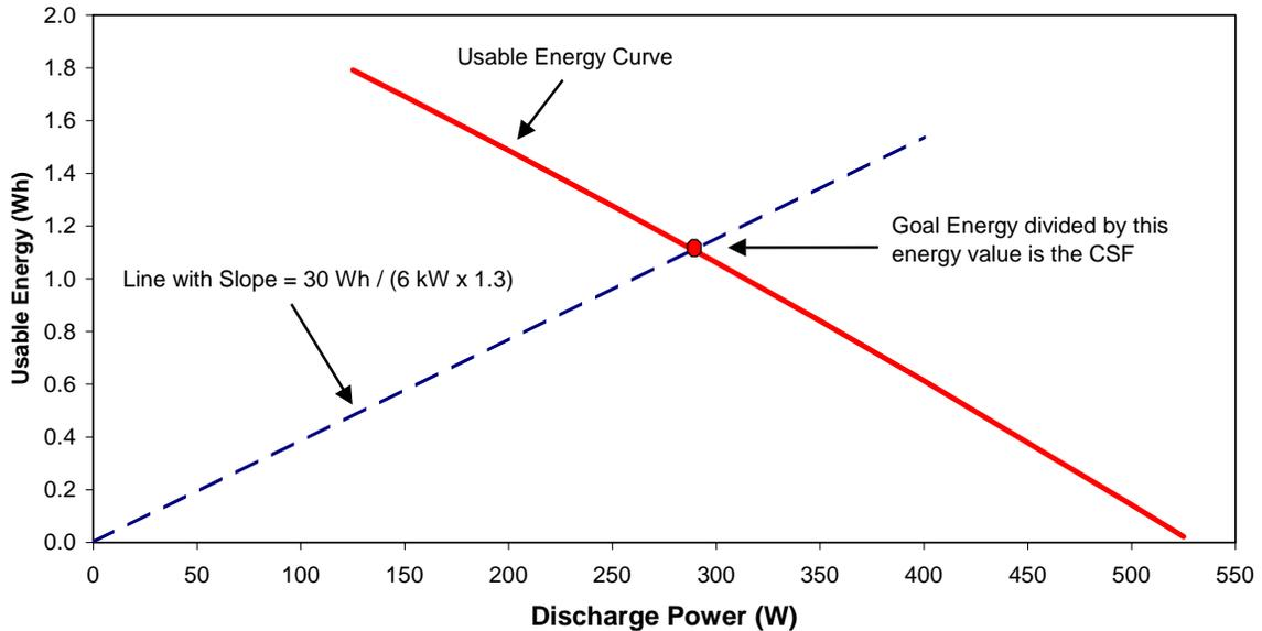
**Figure 29. Finding a Capacitor Size Factor Using Device-Level Results.**
