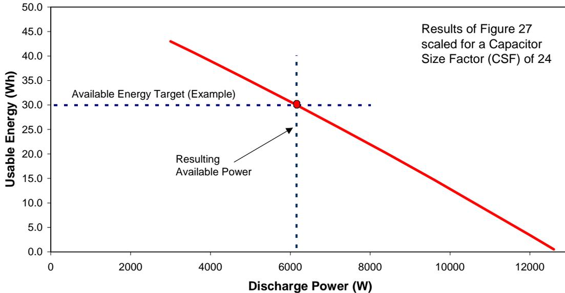
**Figure 28. Determining System Available Power for a System Available Energy Goal of 30 Wh with CSF = 24**
