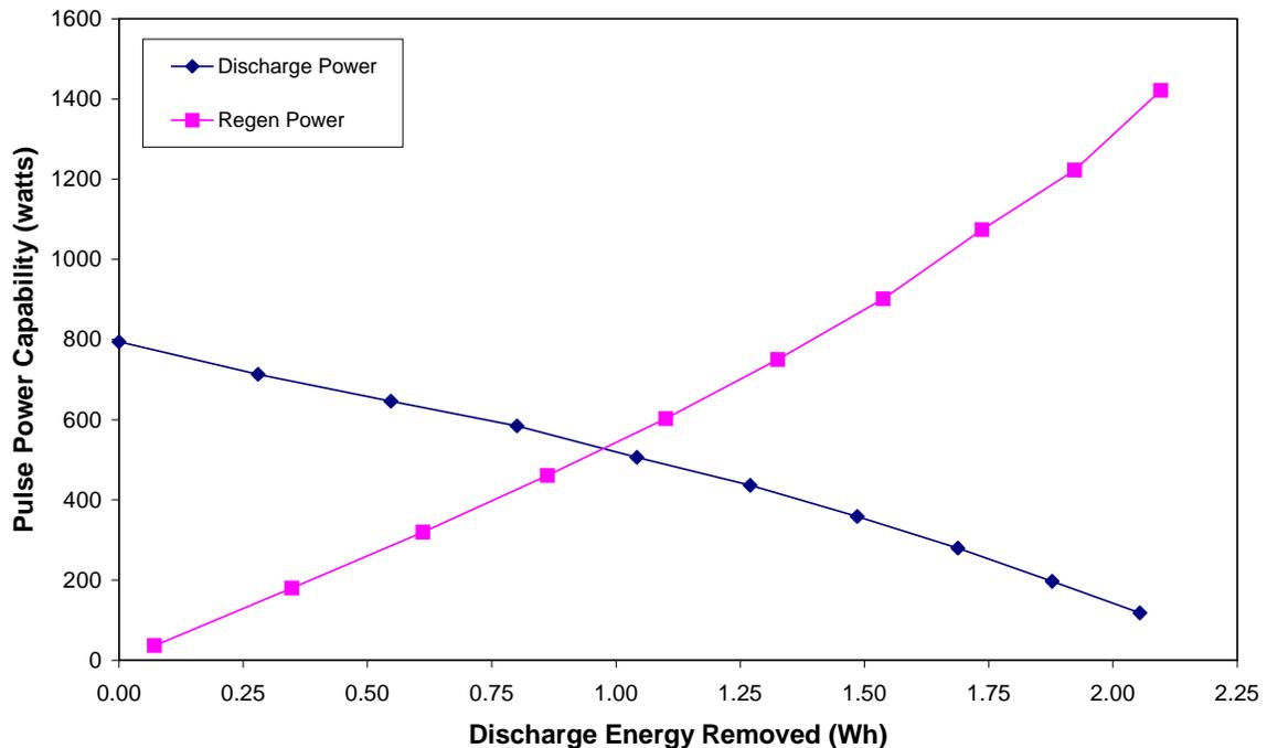
**Figure 24. HPPC Power Capability versus Energy Removed for the data presented in Figures 19 and 23 (unscaled).**
