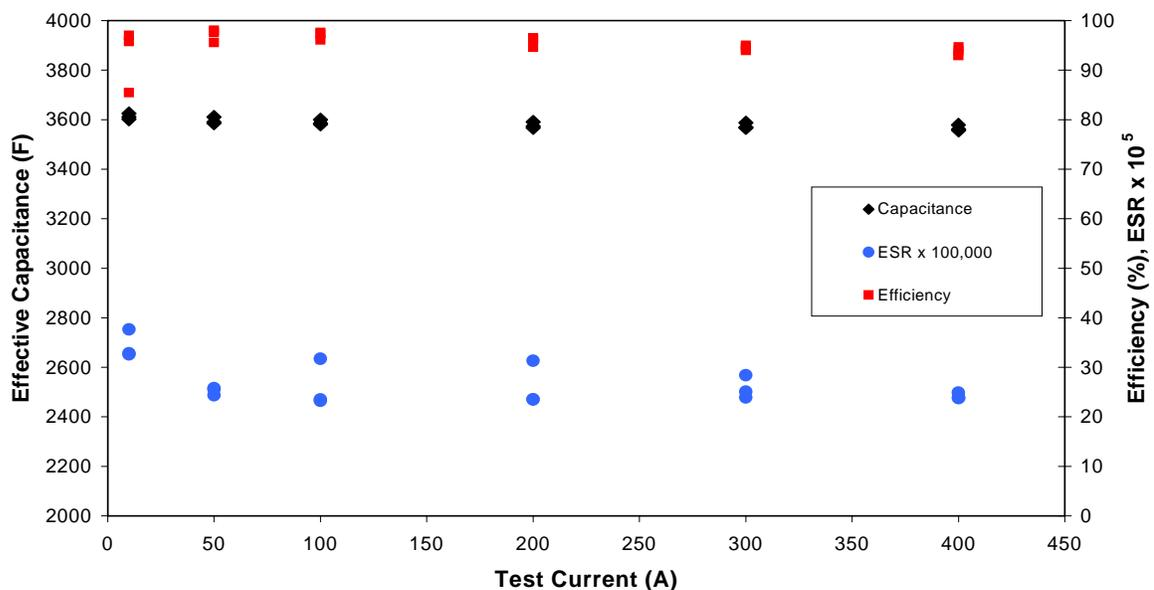
**Figure 9. Cell discharge ESR, effective capacitance and efficiency for a series of constant-current tests.**
