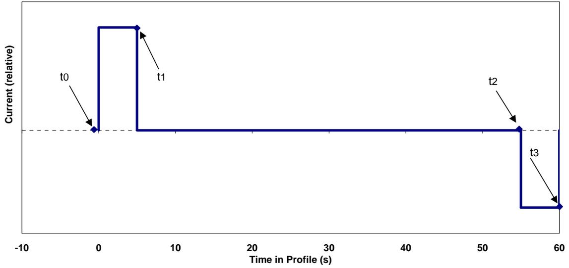
**Figure 20. Resistance Calculation Points for HPPC Pulse Profile**
