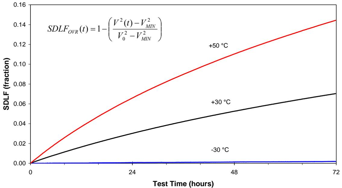
**Figure 16. Self-Discharge Energy Loss Factor calculated from the data of Figure 15.**
