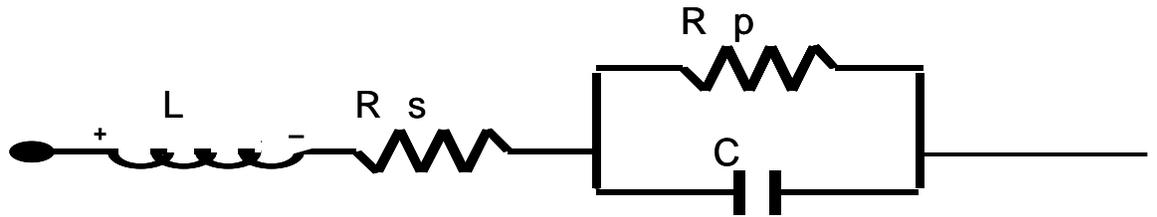
**Figure 1A.** The first-order circuit model of a capacitor. Each of the four circuit elements is ideal.
