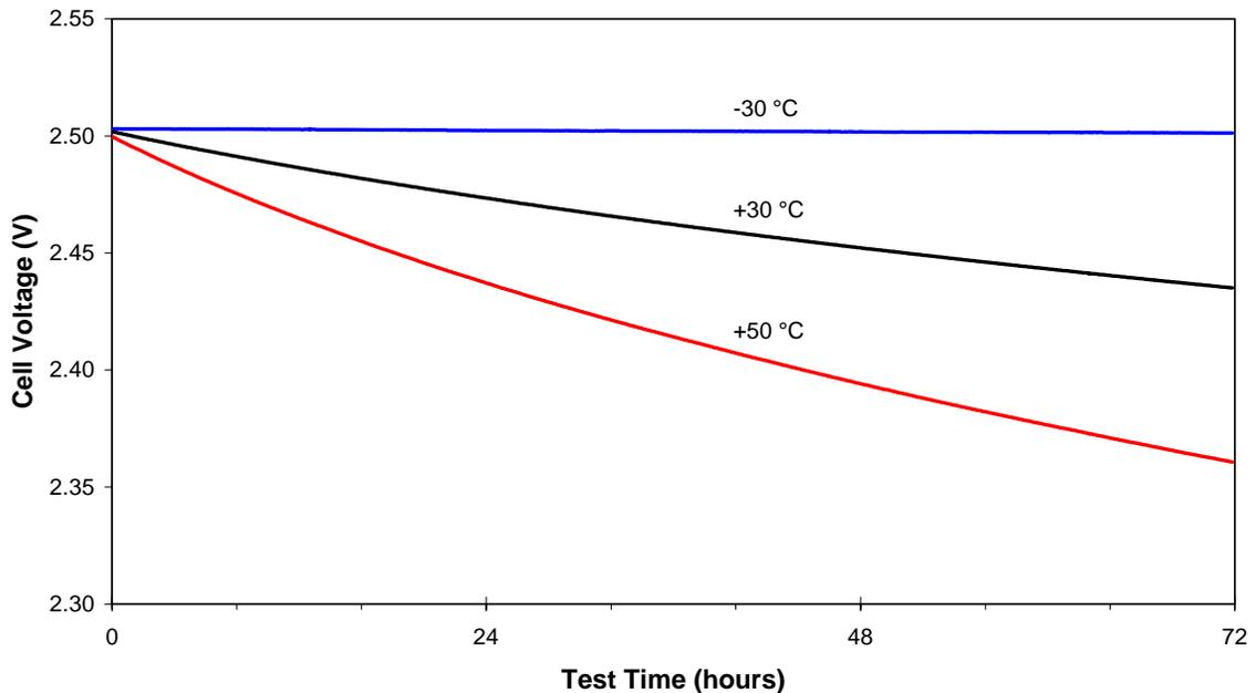
**Figure 15. Cell voltage during a Self-Discharge Test measured at several temperatures.**
