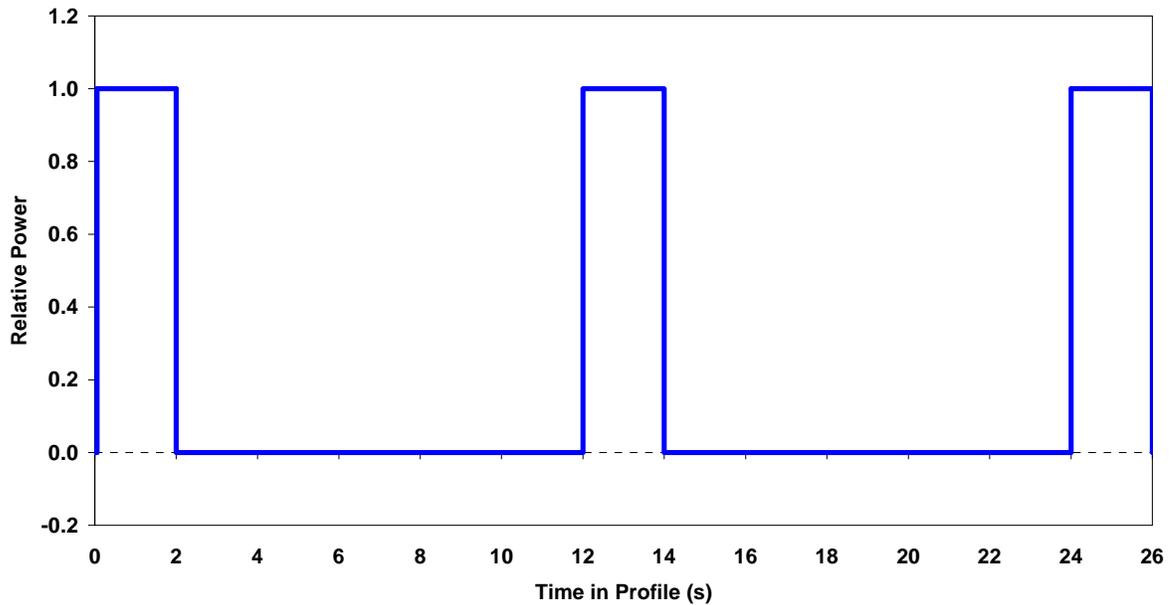
**Figure 4. Cold Cranking Test Profile**
