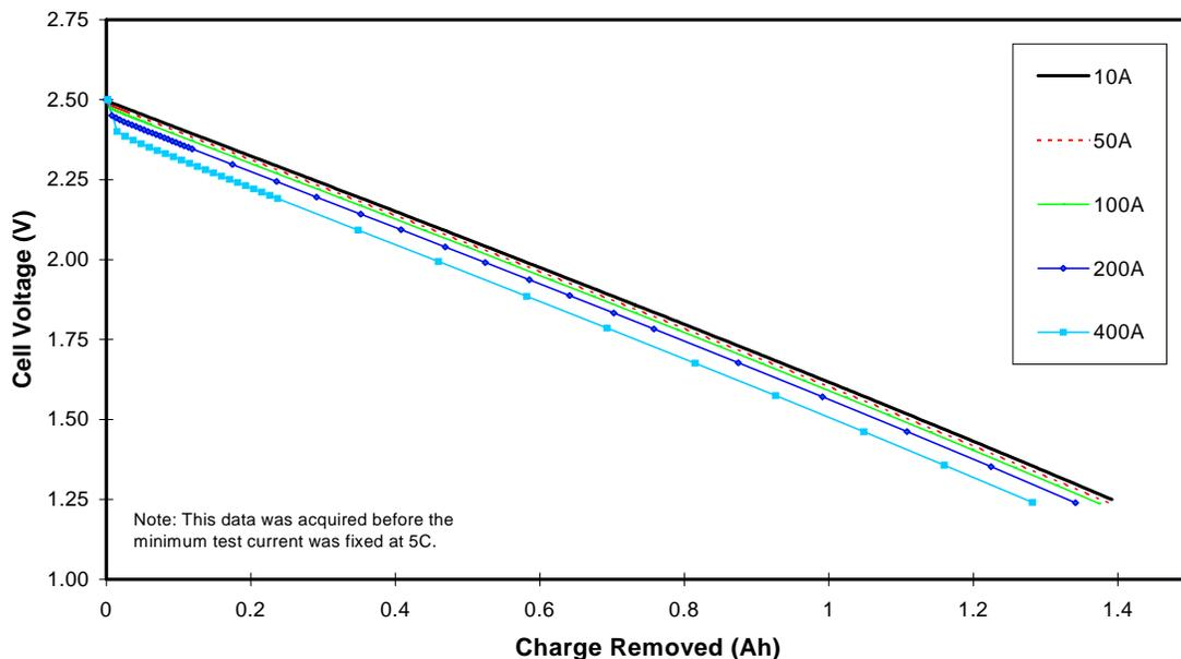
**Figure 7. Cell voltage as a function of charge removed for a series of constant-current tests.**
