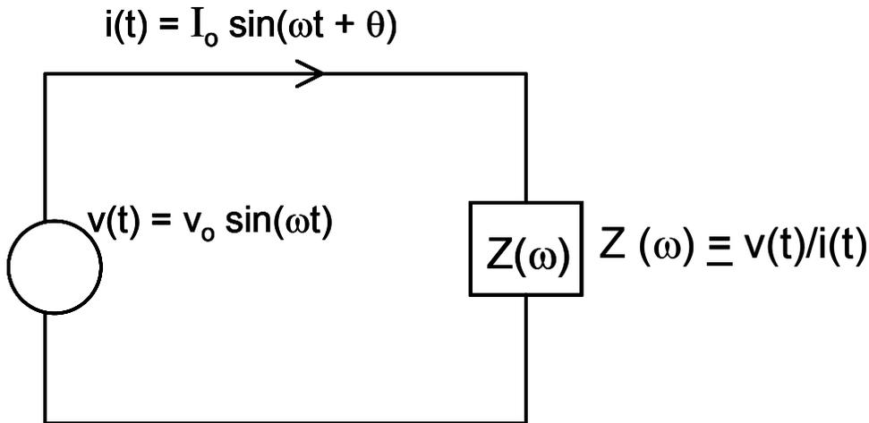
**Figure 1C.** Experimental setup for EIS measurements.
