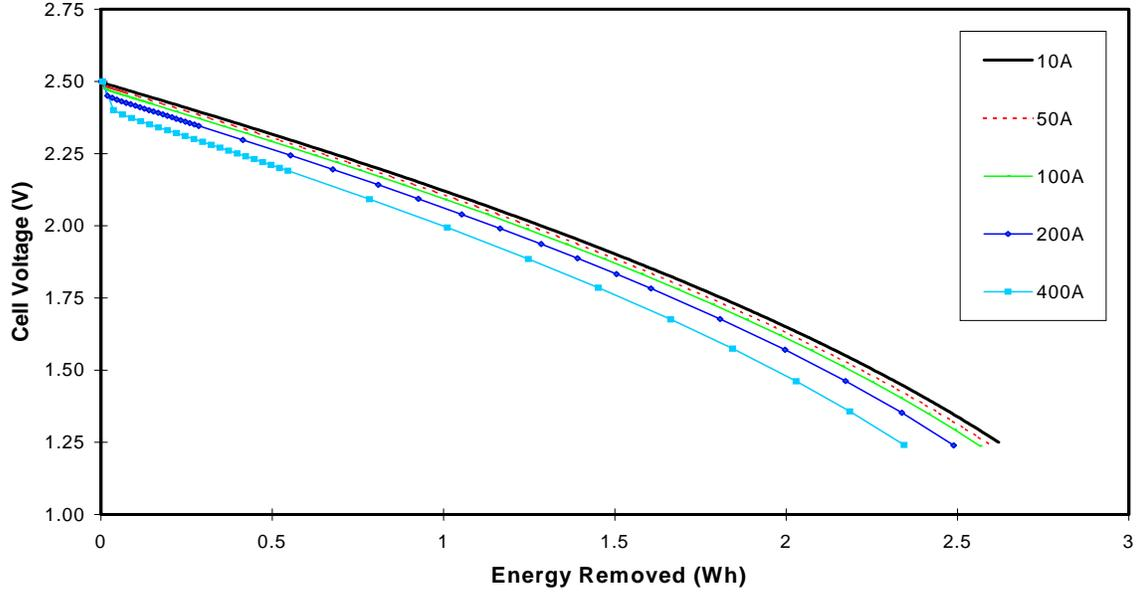
**Figure 8. Cell voltage as a function of the energy removed for a series of constant-current tests.**
