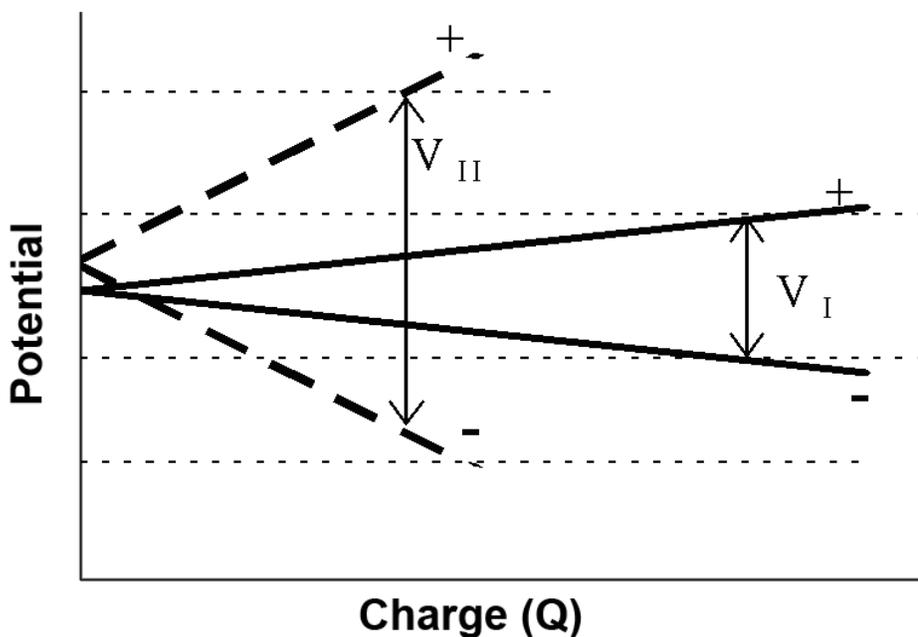
**Figure A-2.** Electrode potentials for an aqueous symmetric Generation I (solid) and an organic symmetric Generation II (dashed) electrochemical capacitor during application of charge  $Q$ .
