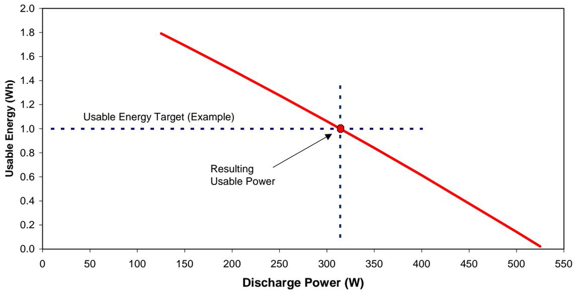
**Figure 27. Determination of Usable Power at a Selected Usable Energy Target**
