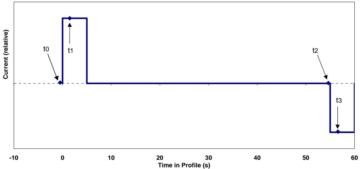
**Figure 22. Resistance Calculation Points (2 s Pulse Capability Example)**
