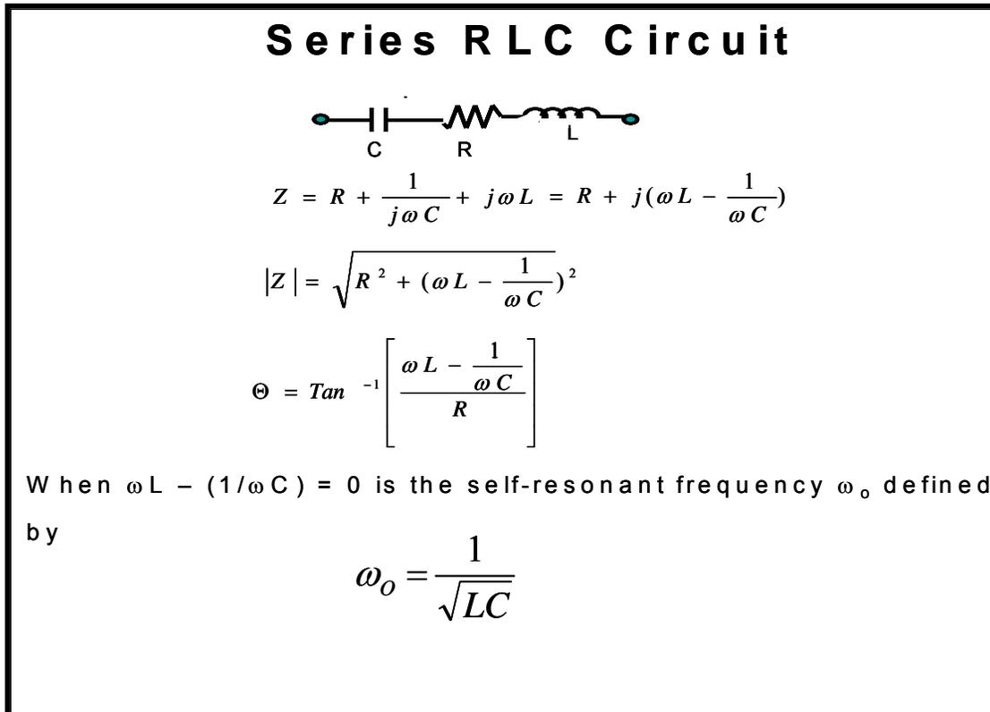
**Figure 2C.** Series RLC circuit model for a two terminal device.
