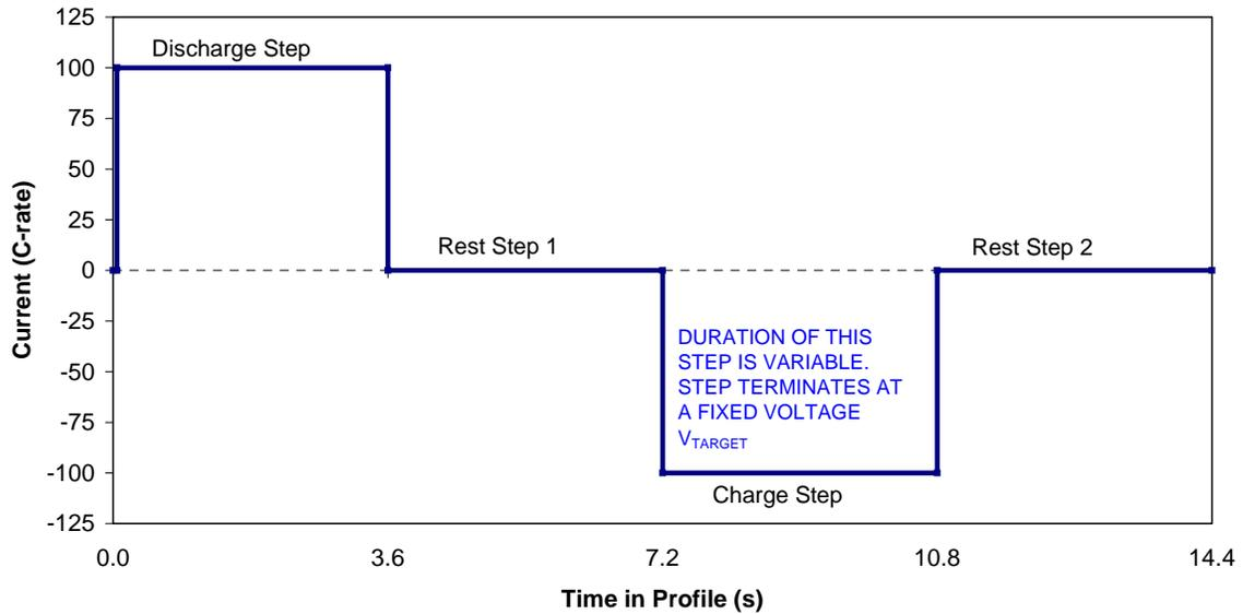
**Figure 5. Ultracapacitor Energy Efficiency and Life Test Profile**
