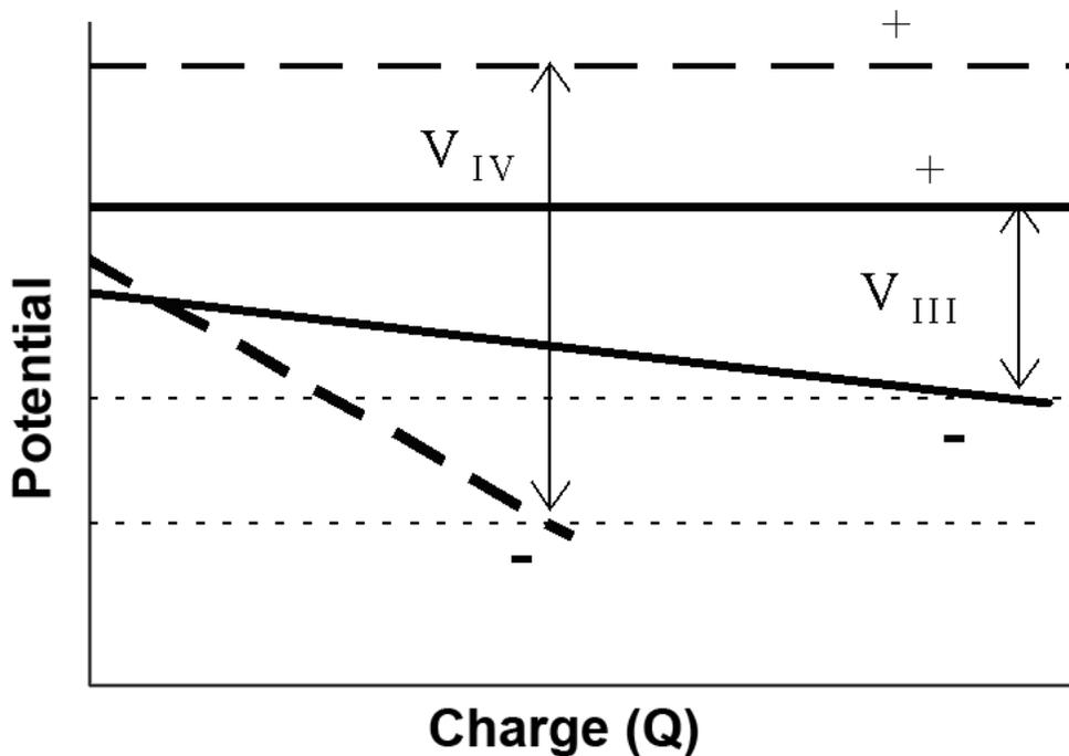
**Figure A-3.** Electrode potentials for a Generation III (solid) and Generation IV (dashed) electrochemical capacitor during application of charge  $Q$ .
