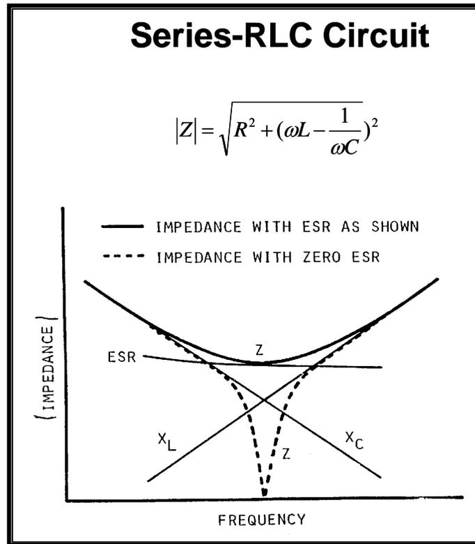
**Figure 3C.** Magnitude of the impedance as a function of frequency.
