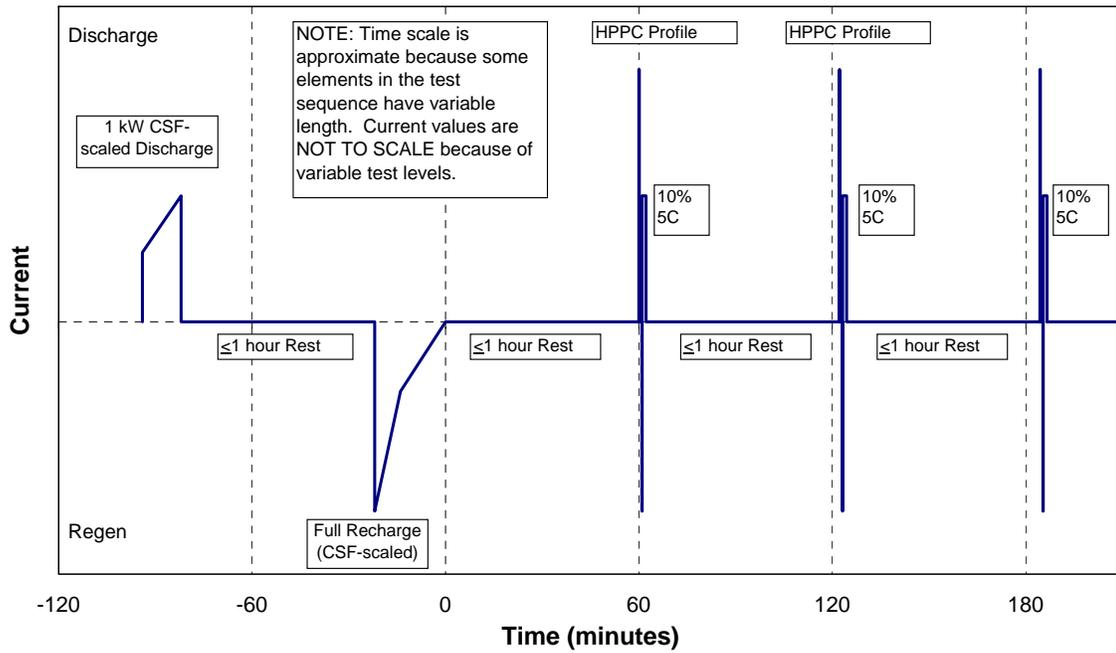
Figure 2. Start of HPPC Test Sequence
