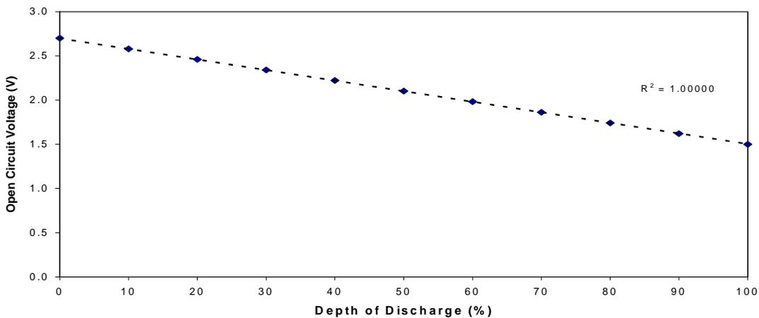
Figure 18. Open Circuit Voltage versus DOD for an Example HPPC Test
