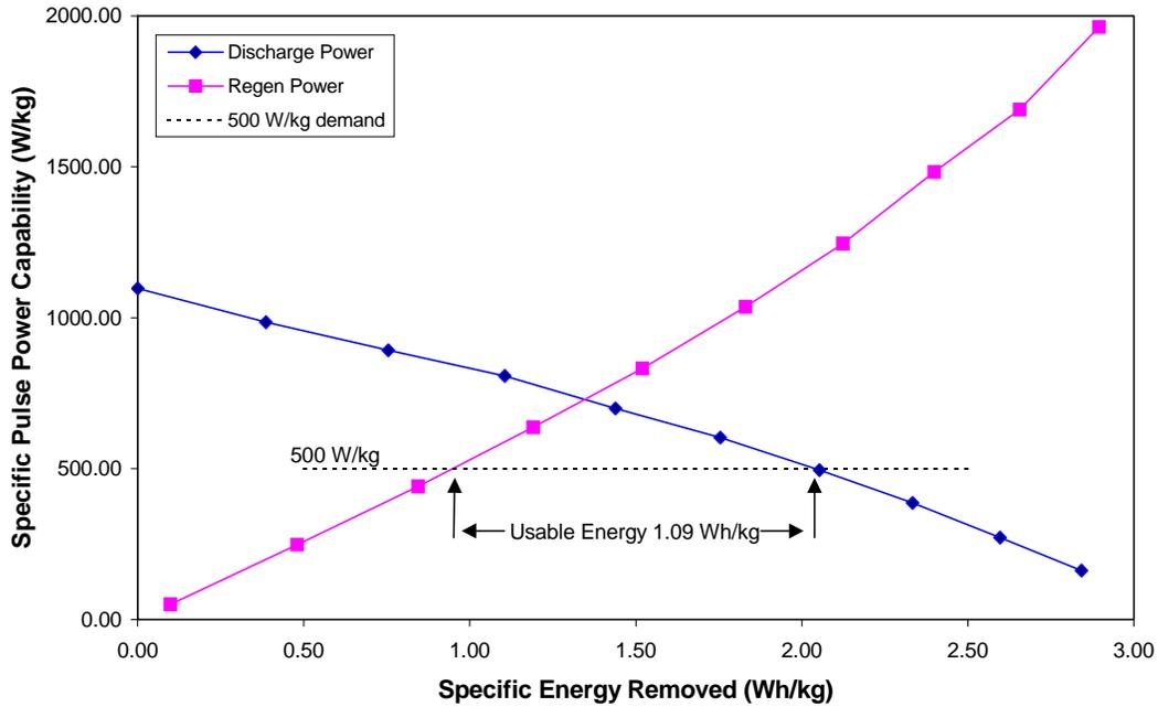
**Figure 25. Specific Energy versus Specific Pulse Power Capability for an Example Ultracapacitor, showing Usable Energy at 500 W/kg**
