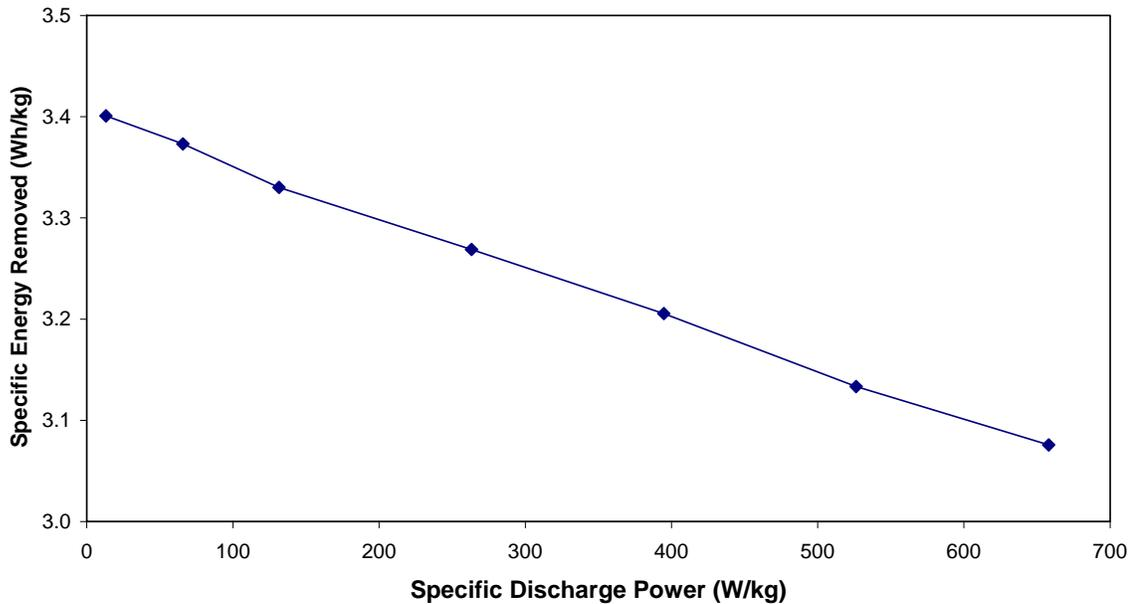
**Figure 11. Specific Energy versus Specific Power for a Representative Ultracapacitor**
