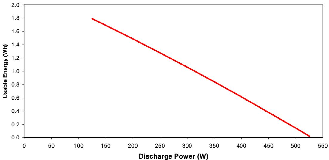
**Figure 26. Example Usable Energy versus Discharge Pulse Power Capability for an Example Capacitor (Unscaled)**
