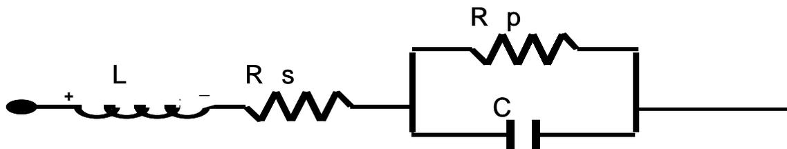
**Figure A-1.** The first-order circuit model of a capacitor. Each of the four circuit elements is ideal.
