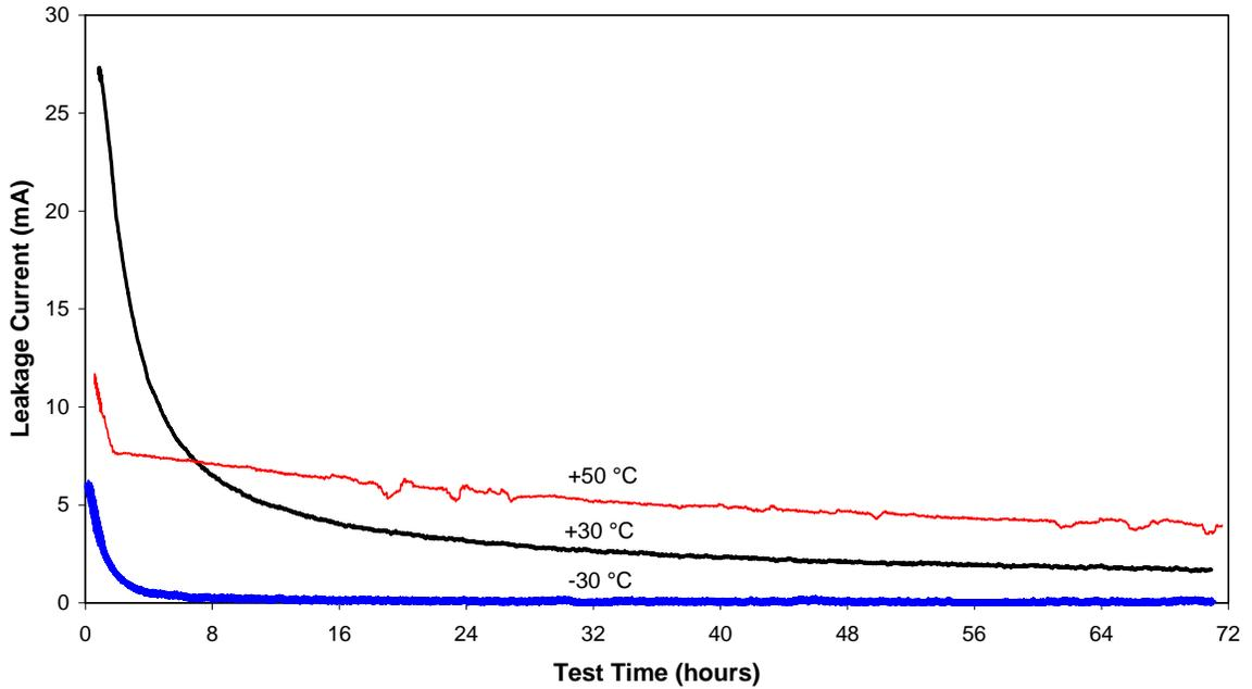
**Figure 12. Leakage current measured on a capacitor at three temperatures.**
