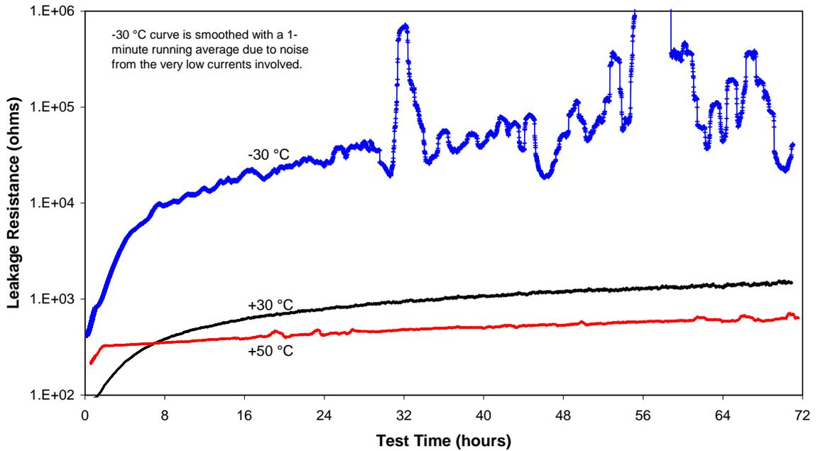
**Figure 13. Leakage resistance determined from data in Figure 12 for a capacitor at three temperatures.**
