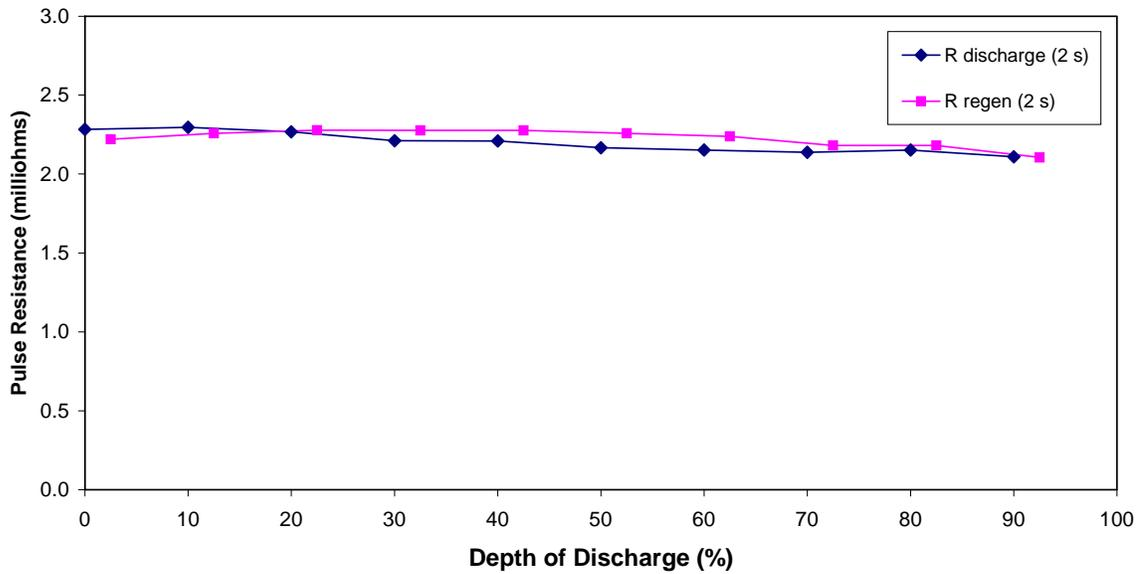
**Figure 21. Discharge and Regen Pulse Resistances for an HPPC Test**
