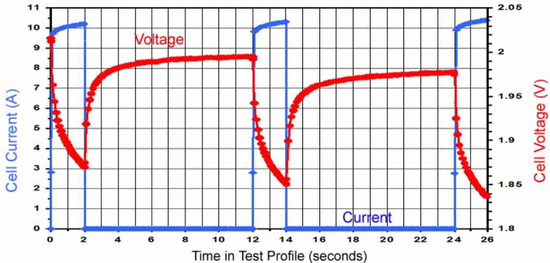
**Figure 31. Example Cold Cranking Discharge Current and Voltage**
