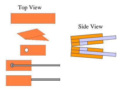
Figure A1. Construction of the test cell. (Not to scale.)
