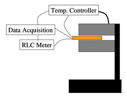
Figure 1. Experimental Arrangement for Shutdown Temperature Test.
