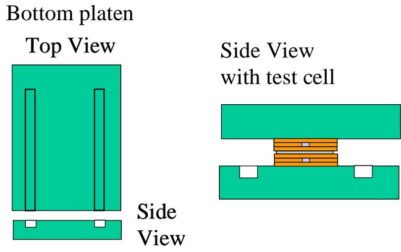
**Figure A2.** Bottom steel plate to hold test cell and RTDs. (Not to scale.)
